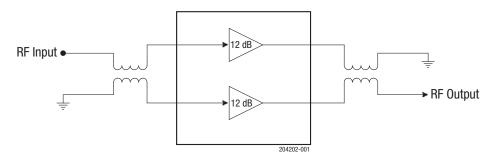
Figure 1. ACA1212 Block Diagram
