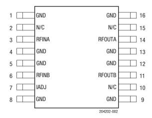
Figure 2. ACA1212 Pinout (Top View)
