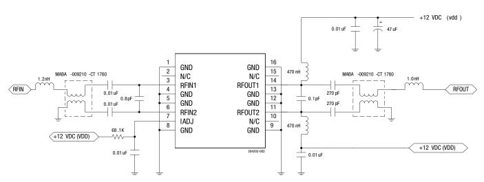
Figure 3. ACA1212 Evaluation Board Schematic
