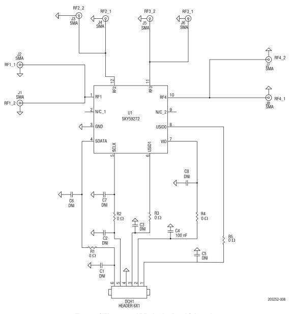
Figure 6. SKY59272-707LF Evaluation Board Schematic
