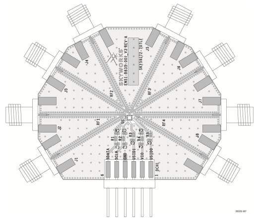
Figure 7. SKY59272-707LF Evaluation Board Assembly Diagram
