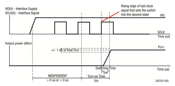
Figure 5. Recommended MIPI Time Sequence Diagram
