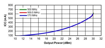
Figure 6. Icc vs Pout, CW
