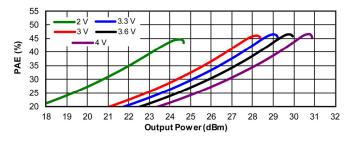
Figure 7. PAE vs Pout and Vcc, CW
