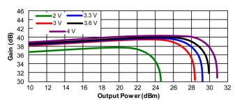
Figure 8. Gain vs Pout and Vcc, CW
