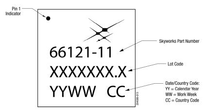
Figure 13. Typical Part Marking
