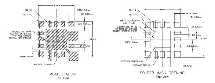
NOTE: THERMAL VIAS SHOULD BE RESIN FILLED AND CAPPED IN ACCORDANCE WITH IPC-4761 TYPE VII VIAS. 30-35UM Cu THICKNESS IS RECOMMENDED.
