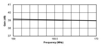
Figure 5. Small Signal Gain vs Frequency, CW
