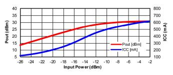
Figure 3. Pout and Icc vs PIN, CW
