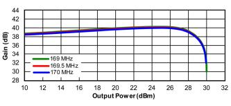
Figure 4. Gain vs Pout, CW
