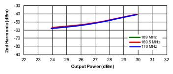
Figure 9. Second Harmonic vs Pout, CW
