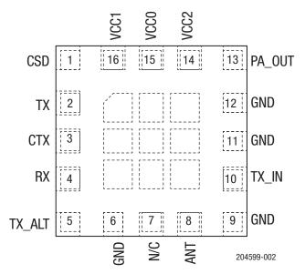
Figure 2. SKY66121-11 Pinout (Top View)
