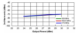
Figure 10. Third Harmonic vs Pout, CW
