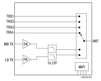
Figure 1. SKY68031-11 Functional Block Diagram
