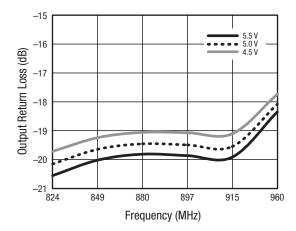
Figure 40. Output Return Loss vs Frequency Over VCC
