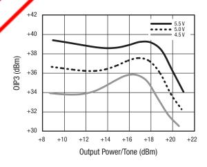
Figure 49. OIP3 vs Output Power/Tone Over VCC
