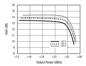
Figure 50. Gain vs Output Power Over Temperature
