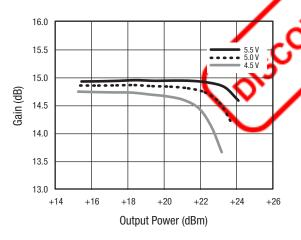
Figure 15. Gain vs Output Power Over VCC
