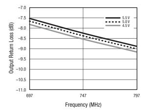
Figure 7. Output Return Loss vs Frequency Over VCC
