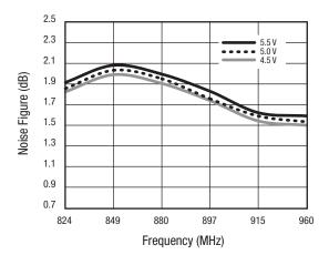
Figure 46. Noise Figure vs Frequency Over VCC
