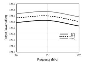
Figure 12. P1dB vs Frequency Over Temperature
