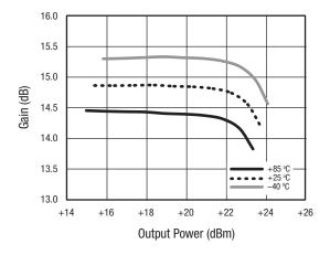
Figure 17. Gain vs Output Power Over Temperature
