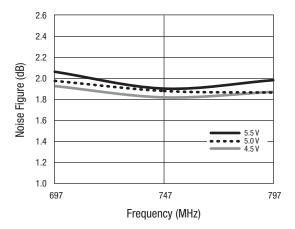
Figure 13. Noise Figure vs Frequency Over VCC
