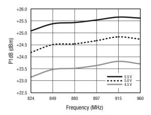
Figure 44. P1dB vs Frequency Over VCC
