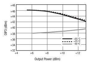
Figure 24. OIP3 vs Output Power Over Temperature
