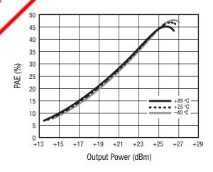
Figure 55. PAE vs Output Power Over Temperature
