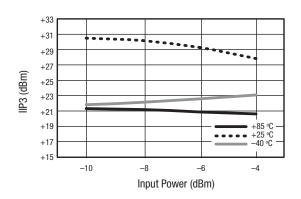
Figure 23. IIP3 vs Input Power Over Temperature
