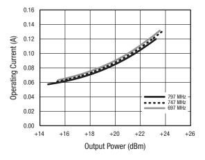
Figure 35. Operating Current vs Output Power Over Frequency
