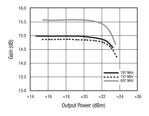
Figure 19. Gain vs Output Power Over Frequency
