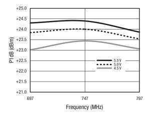
Figure 11. P1dB vs Frequency Over VCC
