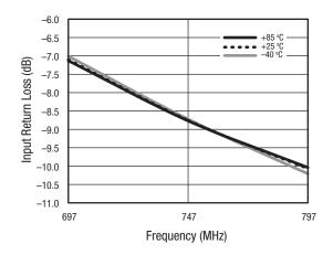
Figure 5. Input Return Loss vs Frequency Over VCC
