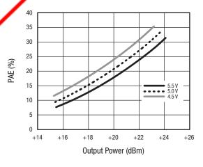
Figure 16. PAE vs Output Power Over VCC
