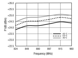
Figure 45. P1dB vs Frequency Over Temperature
