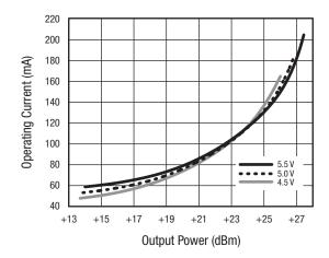
Figure 57. Operating Current vs Output Power Over VCC
