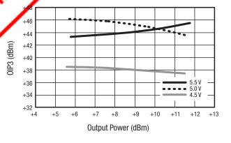
Figure 22. OIP3 vs Output Power Over VCC
