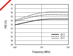
Figure 27. PAE @ P1dB vs Frequency Over VCC
