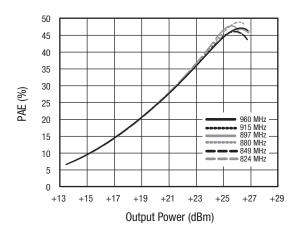
Figure 56. PAE vs Output Power Over Frequency
