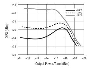
Figure 51. 0IP3 vs Output Power/Tone Over Temperature
