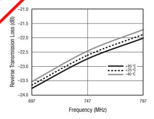
Figure 10. Reverse Transmission Loss vs Frequency Over **Temperature**
