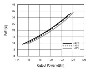
Figure 18. PAE vs Output Power Over Temperature
