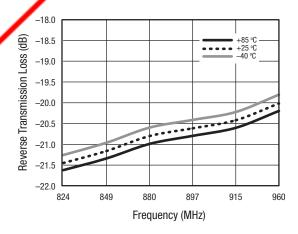
Figure 43. Reverse Transmission Loss vs Frequency Over **Temperature**
