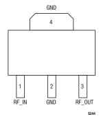
Figure 1. SKY65045-70LF Pinout Package (Top View)
