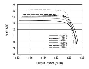
Figure 52. Gain vs Output Power Over Frequency
