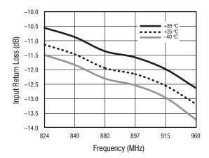
Figure 38. Input Return Loss vs Frequency Over VCC
