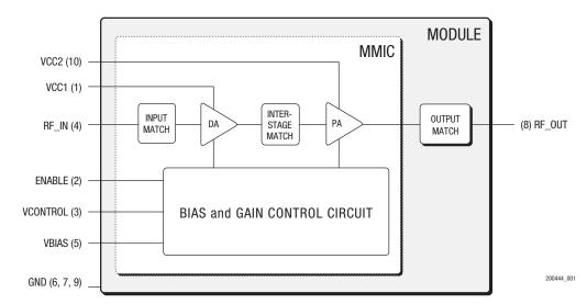
Figure 1. SKY77174 Functional Block Diagram
