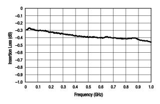
**Figure 3. Typical Insertion Loss**
