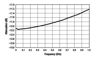
Figure 5. Typical Attenuation (Normalized to Insertion Loss)
