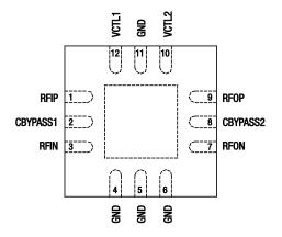
Figure 2. SKY12407-321LF Pinout – 12-Pin QFN (Top View)
