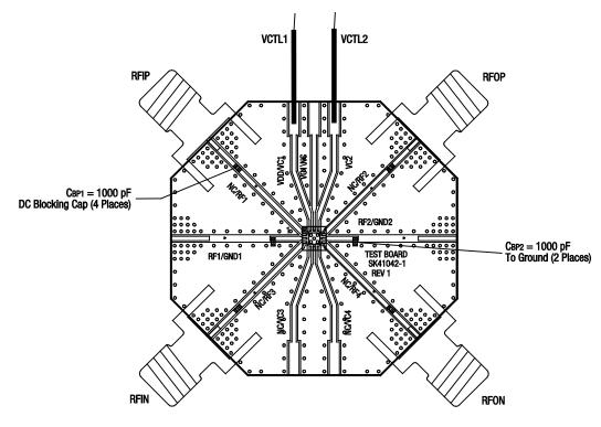
Figure 7. SKY12407-321LF Evaluation Board Assembly Diagram
