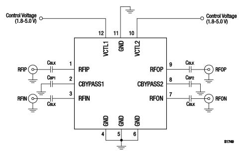
Figure 8. SKY12407-321LF Evaluation Board Schematic Diagram
