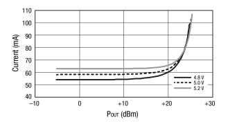
Figure 12. Current vs Output Power Over Voltage
