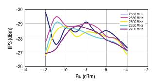
**Figure 8. IIP3 vs Input Power Over Frequency**
