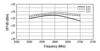
Figure 10. OP1dB vs Frequency Over Voltage
