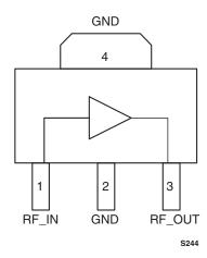
Figure 2. SKY65081-70LF Pinout (Top View)
