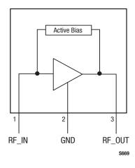
Figure 1. SKY65081-70LF Functional Block Diagram
