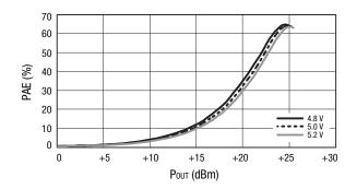
Figure 11. PAE vs Output Power Over Voltage
