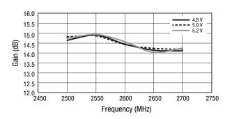
Figure 4. Gain vs Frequency Over Voltage
