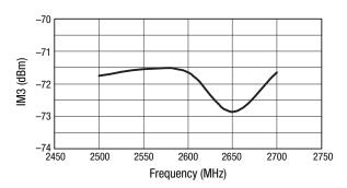
Figure 7. IM3 vs Frequency (PiN = -10 dBm)
