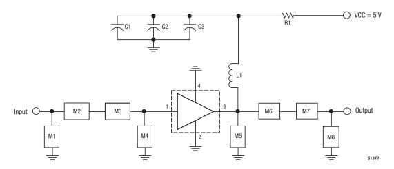
Figure 15. SKY65081-70LF Evaluation Board Schematic (2500 MHz to 2700 MHz, IIP3 Matched)
