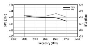
Figure 6. OIP3 vs Frequency
