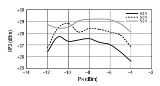
Figure 9. IIP3 vs Input Power Over Voltage
