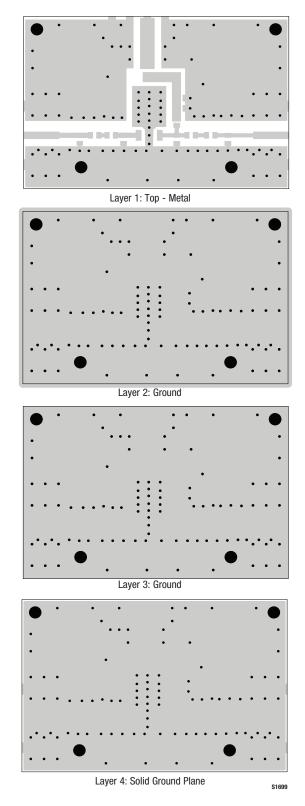
Figure 14. Evaluation Board Layer Detail
