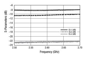
Figure 3. Return Loss vs Frequency
