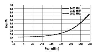
Figure 13. Detector Voltage vs Output Power Over Frequency
