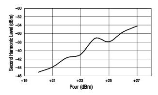
Figure 17. Second Harmonic vs Output Power (802.11b)
