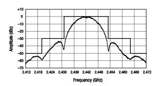
Figure 16. Spectral Response @ Pout = +31 dBm (802.11b, CCK @ 11 Mbps)
