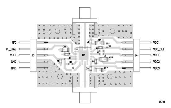
Figure 19. SKY65135-31 Evaluation Board Assembly Diagram
