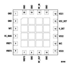
Figure 2. SKY65135-31 Pinout – 20-Pin MCM (Top View)
