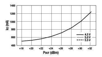
Figure 12. Supply Current vs Output Power Over Vcc
