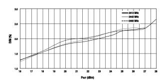
**Figure 7. EVM vs Output Power Over Frequency**
