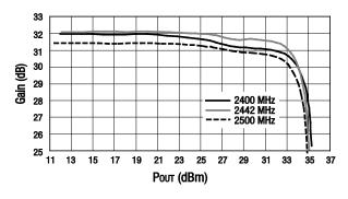
**Figure 3. Gain vs Output Power Over Frequency**
