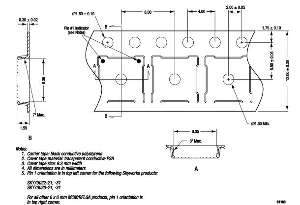
Figure 25. SKY65135-31 20-Pin MCM Tape and Reel Dimensions
