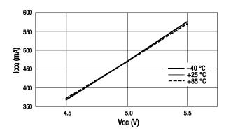
Figure 9. Quiescent Current vs Vcc Over Temperature
