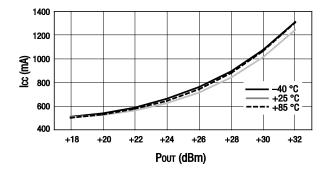
Figure 10. Current vs Output Power Over Temperature @ 5 V
