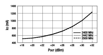
**Figure 11. Supply Current vs Output Power Over Frequency**
