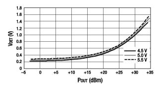
Figure 14. Detector Voltage vs Output Power Over Vcc
