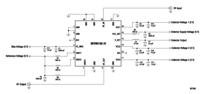
Figure 18. SKY65135-31 Evaluation Board Schematic
