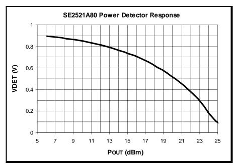
Figure 3: SE2521A80 Power Detector Performance Curve
