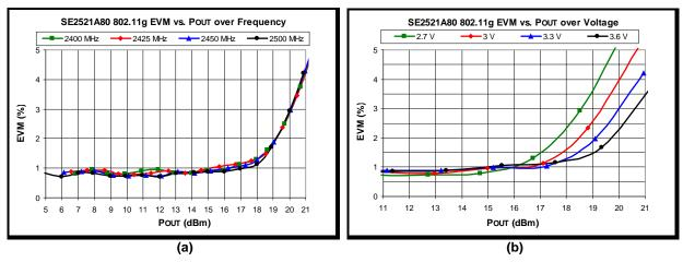
Figure 4: SE2521A80 802.11g 54 Mbps EVM vs. Pout (a) Over Frequency (b) Over Voltage
