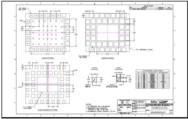
Figure 8: SE2521A80 Recommended PCB Footprint
