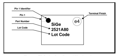
Figure 9: SE2521A80 Branding and Pin 1 Location
