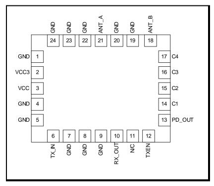
Figure 2: SE2521A80 Pin-Out (Top View Through Package)
