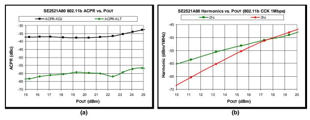
Figure 5: SE2521A80 802.11b Performance (a) ACPR vs. Pout, (b) Harmonics vs. Pout
