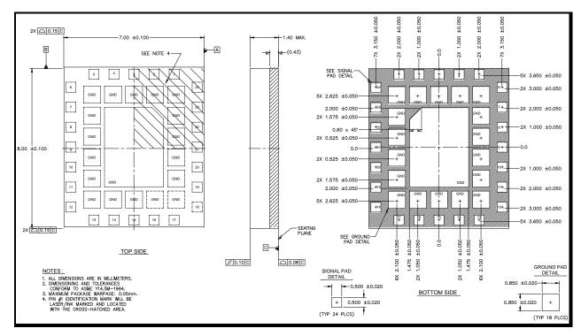
Figure 7: SE2521A80 Package Diagram
