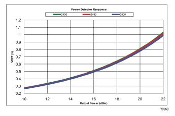
Figure 3. SE2611T Power Detector Characteristics
