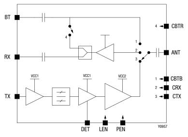
Figure 2. SE2611T Block Diagram
