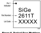
**Figure 5. Typical Case Markings** (Top View)
