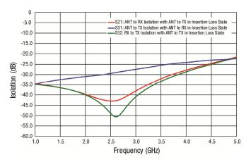
Figure 4. Isolation vs Frequency
