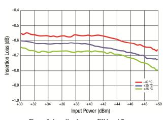
Figure 6. Insertion Loss vs CW Input Power (TX to ANT Port, f = 2600 MHz, 28 V, 100 mA, EVB Loss Included)
