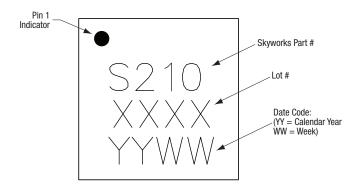
Figure 17. Typical Part Markings
