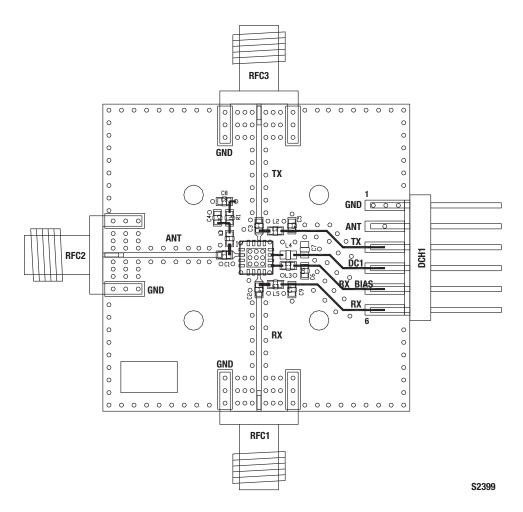
Figure 13. SKY12210-478LF Evaluation Board Assembly Diagram
