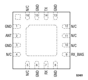
Figure 2. SKY12210-478LF Pinout (Top View)
