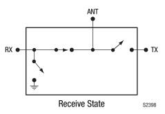
Figure 12. SKY12210-478LF Equivalent Circuit Diagrams
