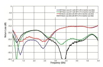
Figure 5. Return Loss vs Frequency
