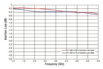
**Figure 3. Insertion Loss vs Frequency**
