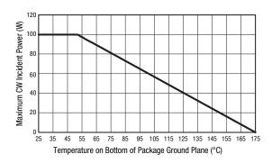
Figure 10. Transmit Power Derating, Maximum CW Incident Power (Frequency = 2.6 GHz) vs Ground Plane Temperature
