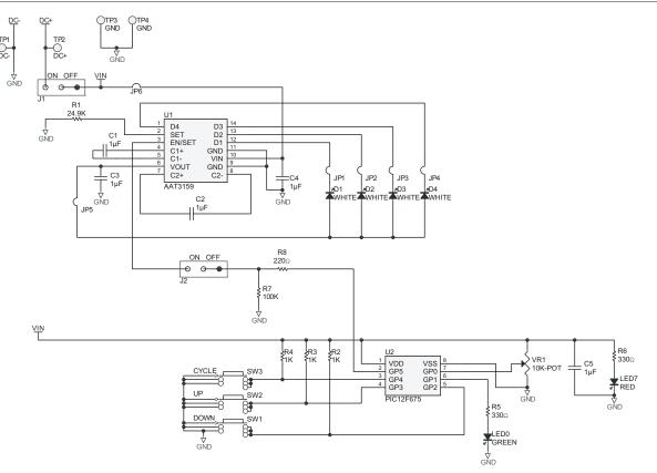
Figure 4: AAT3159 Evaluation Board Schematic.
