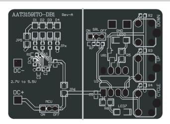
Figure 5: AAT3159 Evaluation Board Top Side Layout.
