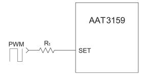
Figure 3: SET Pin Configuration for PWM Dimming Control.
