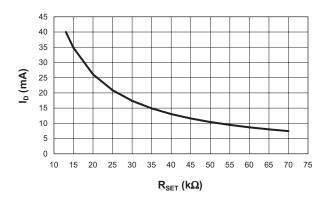
Figure 1: Maximum LED Current vs. R<sub>SET</sub>.
