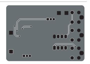
Figure 6: AAT3159 Evaluation Board Bottom Side Layout.
