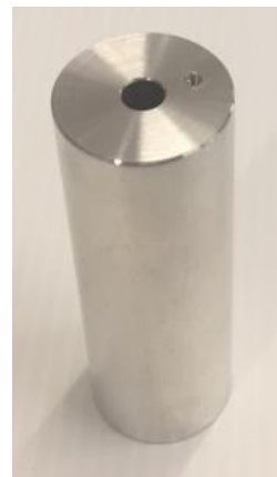
Figure 1. Endpoint booster [2] for enhancement of the standard OES attachment on the ICP chamber.
