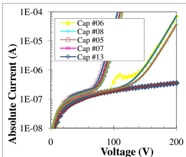
Fig.2. Log-scaled measured and modeled IV curves of five Skyworks ESD Capacitors with different areas. The substrate leakage current from metal pads to the back of the wafer is also listed for comparison
