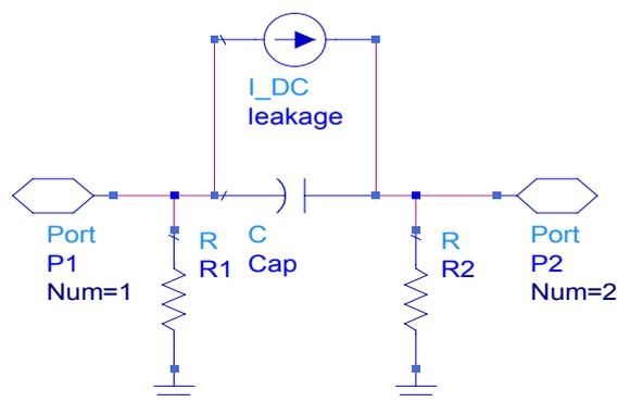
Fig.1. Equivalent circuit schematic of Skyworks ESD Capacitor Model.
