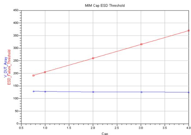
Fig.4. Simulated ESD breakdown voltages of a variety of capacitors and the voltage drop across these capacitors when they explode
