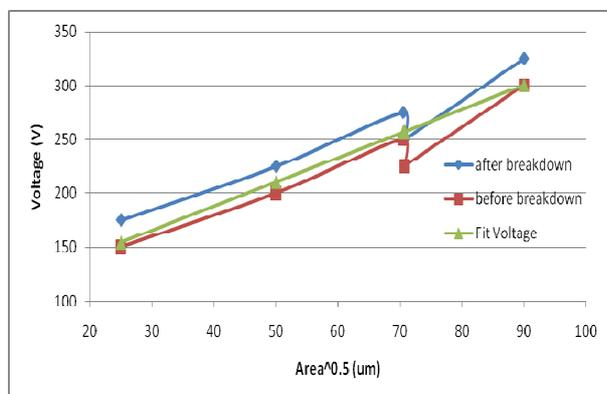
Fig.3. Measured and modeled ESD breakdown voltages of five Skyworks ED capacitors with different areas.
