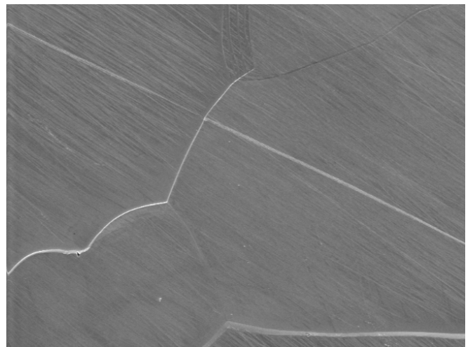
Figure 6 100X SEM image of a clean Au source
