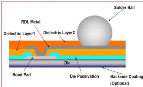
Figure 1: The cross section of RDL Process
