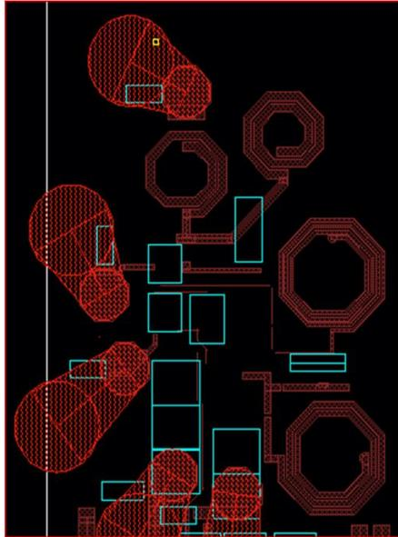
**Figure 4: LNA layout with RDL**
