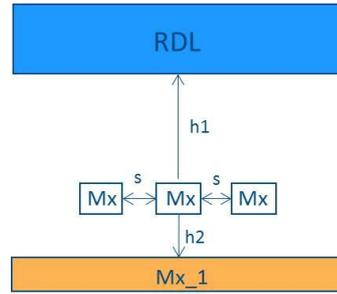
Figure 3: Nested metal line test structure
