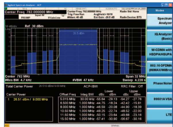
Fig.2 5.2dB SEM Margin at 26.5dBm with 10MHz QPSK 50RB MPR=1 Signal
