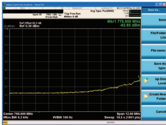
Fig.4 5.8dB NS_07 Margin at 26.5dBm with 10MHz QPSK 16RB MPR=1 Start from 19RB Signal
