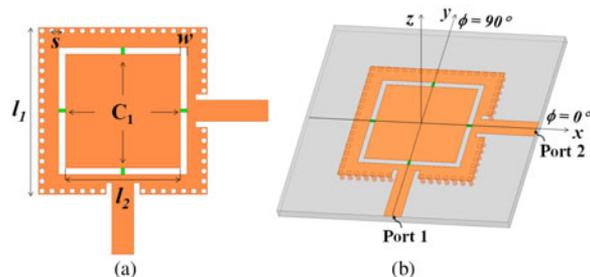
Fig. 1. (a) Top view of the proposed single antenna. (b) Perspective view and coordinators. (Parameters:  $l_1 = 25$  mm,  $l_2 = 17$  mm,  $w = 1$  mm,  $s = 1.5$  mm, and  $C_1 = 3$  pF.)
