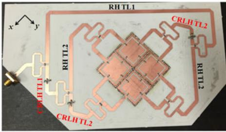
Fig. 8. Photograph of the proposed dual-band circular polarization array antenna.
