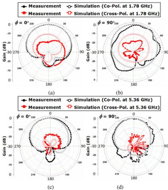
Fig. 6. Normalized gain patterns of the single antenna. The first broadside radiation modes at (a)  $xz$  plane and (b)  $yz$  plane. Normalized gain patterns of the second broadside radiation mode at (c)  $xz$  plane and (d)  $yz$  plane.
