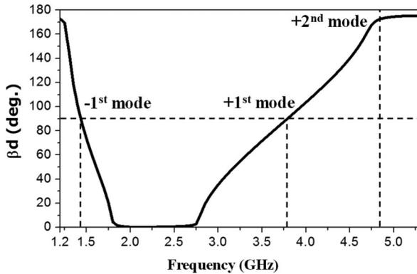
Fig. 3. Dispersion diagram of the fundamental CRLH unit cell.
