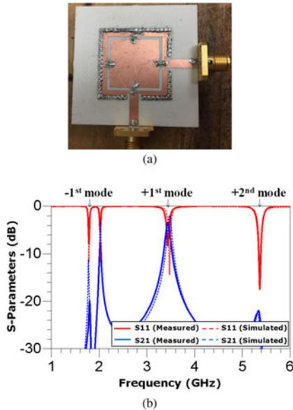
Fig. 5. (a) Photograph of the proposed single antenna. (b)  $S$ -parameters of the proposed single antenna.
