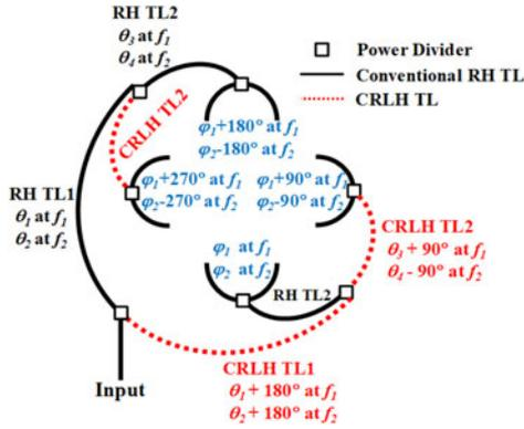
Fig. 7. Operating diagram of the dual-band feeding network for circularly polarized radiations.
