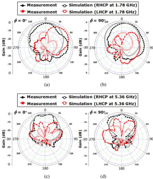
Fig. 9. Normalized gain patterns of the array antenna. The first broadside radiation mode at (a)  $xz$  plane and (b)  $yz$  plane. Normalized gain patterns of the second broadside radiation mode at (c)  $xz$  plane and (d)  $yz$  plane.
