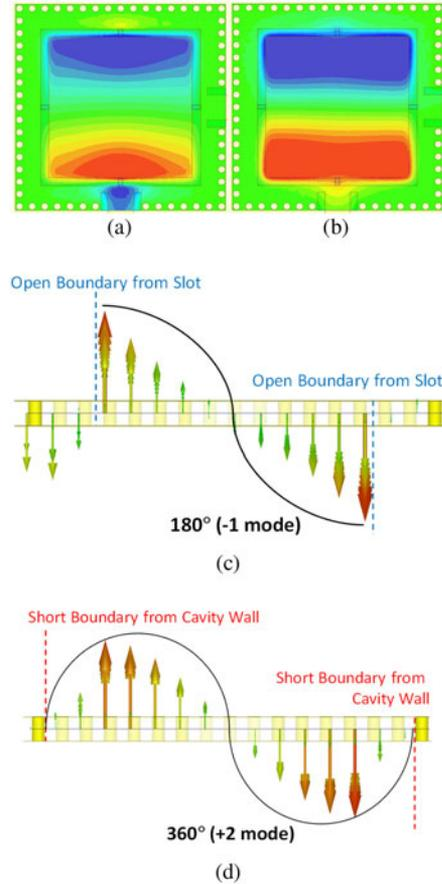
Fig. 4. Z-directed electric field distributions on  $xy$  plane: (a) first broadside radiation mode at 1.78 GHz and (b) second broadside radiation mode at 5.36 GHz. Z-directed electric field distributions on  $yz$  plane: (c) first broadside radiation mode at 1.78 GHz and (d) second broadside radiation mode at 5.36 GHz.
