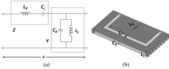
Fig. 2. (a) General circuit diagram of CRLH structure. (b) Fundamental unit cell of the proposed single antenna cavity.
