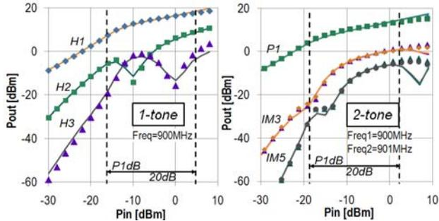
Fig. 3. Large-signal prediction of the full-blown HICUM model versus 1- and 2-tone large-signal characterization data of a  $4 \times 1.2 \mu\text{m} \times 20 \mu\text{m}$  transistor at  $V_{BE}=0.8\text{V}$ ,  $V_{CE}=3.0\text{V}$ . Symbols represent the characterization data; lines the model prediction.
