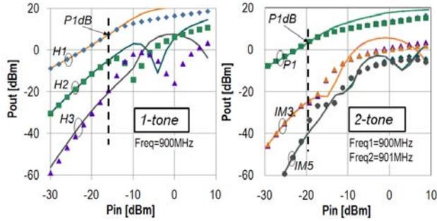
Fig. 2. Prediction of a simple SGPM model versus 1- and 2-tone large-signal characterization data of a  $4 \times 1.2 \mu\text{m} \times 20 \mu\text{m}$  transistor  $V_{BE}=0.8\text{V}$ ,  $V_{CE}=3.0\text{V}$ . Symbols represent the characterization data; lines the model prediction.
