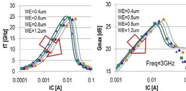
Fig. 1. RF performance,  $f_T$  on the right and  $G_{\text{max}}$  on the left, of transistors of different WE of 0.4, 0.6, 0.8, and  $1.2\mu\text{m}$  and constant  $L_E=20\mu\text{m}$ . Symbols represent the measured data and lines model prediction.
