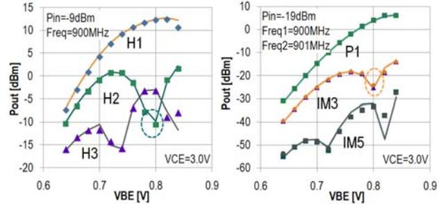
Fig. 4. Large-signal prediction of the full-blown HICUM model versus  $V_{BE}$  for a  $4 \times 1.2 \mu\text{m} \times 20 \mu\text{m}$  transistor at constant  $P_{in}=-9$  and  $-19\text{dBm}$  for 1- and 2-tone characterization; Symbols represent the characterization data; lines the model prediction.
