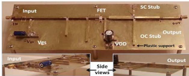
Fig.7. Transmission-line class-E amplifier prototype.
