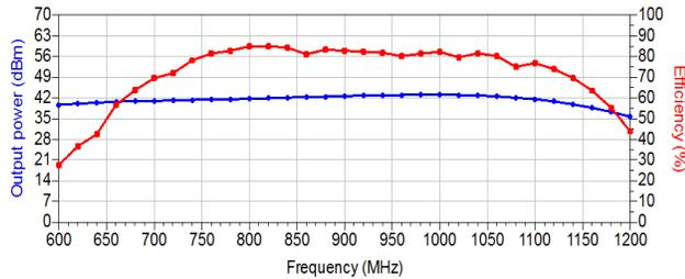
Fig.8. Measured output power and efficiency.
