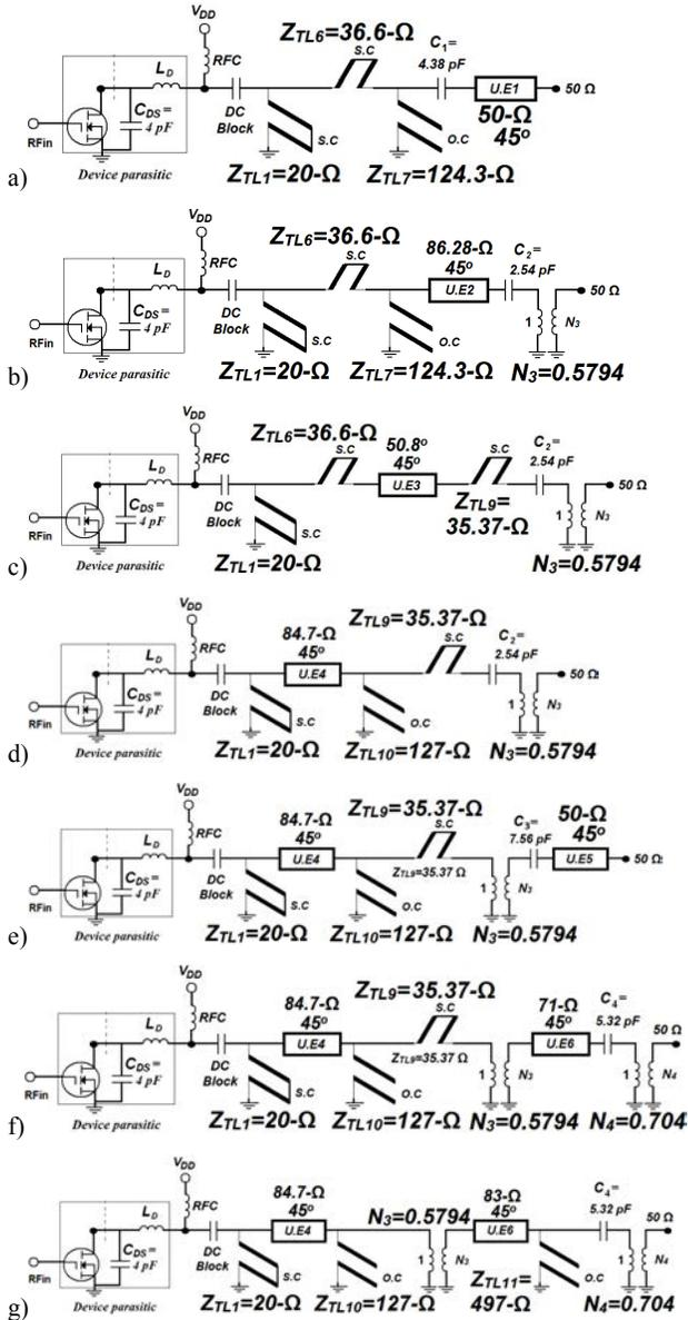
Fig.4. Transformation sequence to obtain shunt-connected wire-lines.
