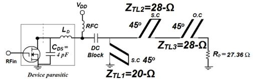
Fig. 1. Wire-line transmission-line class-E PA.
