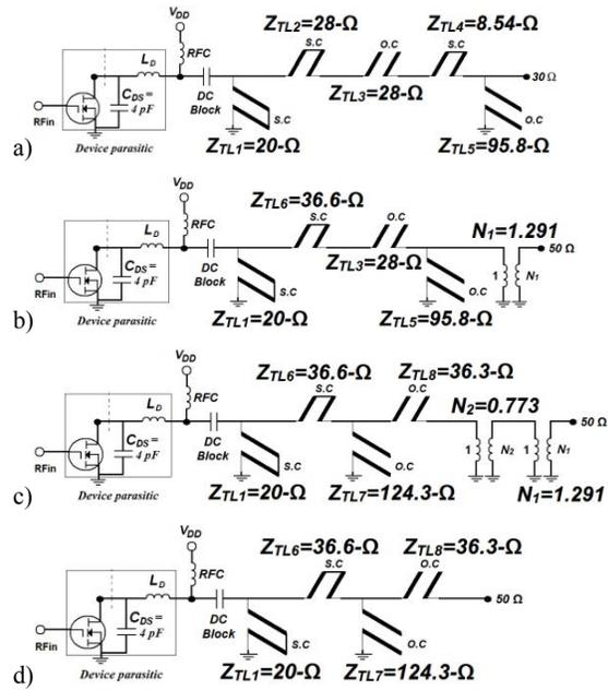
Fig.3. Wire-line transforms. All line lengths are  $45^\circ (1/8\lambda)$ .
