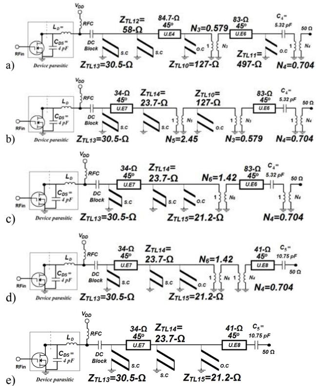
Fig.5. Transformers elimination sequence.
