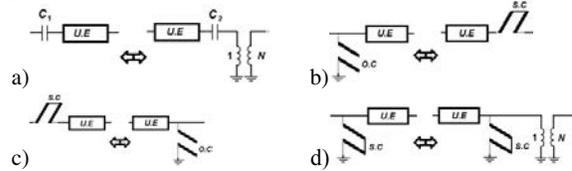
Fig. 2. Richard's transforms. All wire-lines and UE are 45° in length.
