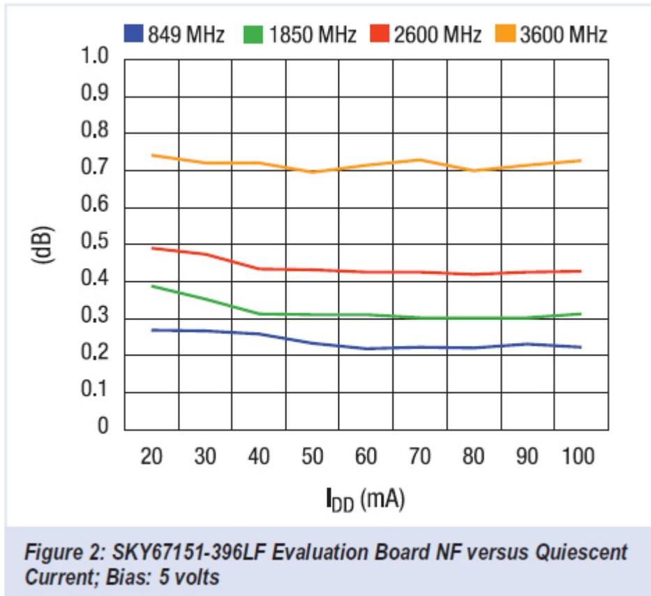
Note the excellent gain and gain flatness over this wide band to go along with the industry leading NF performance. Since the evaluation board losses have not been de-embedded from this data, this NF and gain is representative of the performance the device can achieve on an actual customer system board using an efficient layout.
