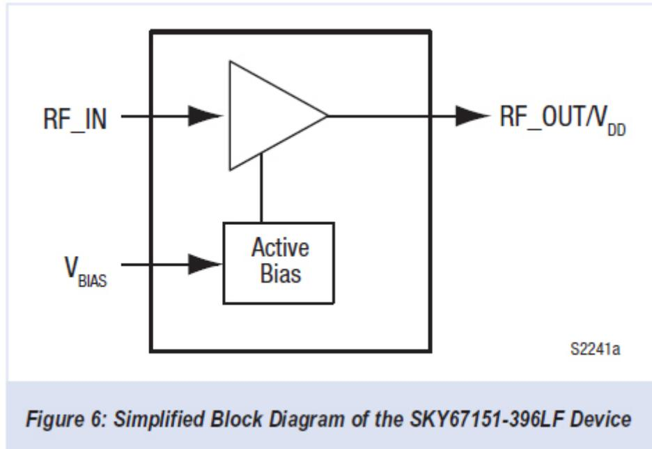
**Figure 6: Simplified Block Diagram of the SKY67151-396LF Device**
