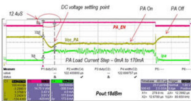
Figure 5: DC-DC voltage regulator load transient response corresponding to a 0 to 170 mA RF PA load step for an 802.11ac transition measured for an RF PA output at 18dBm
