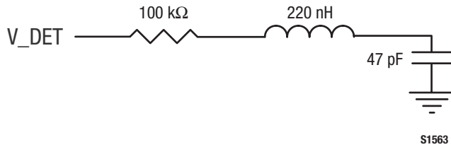
Figure 3. Recommended Notch Filter Topology
