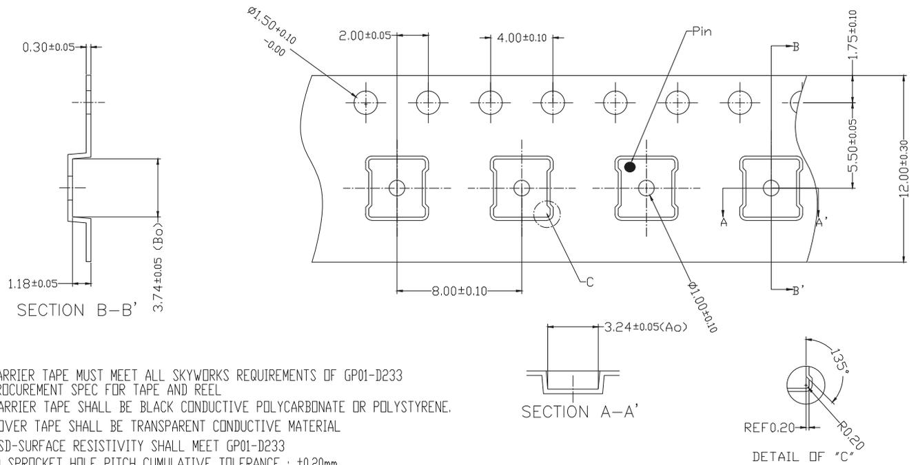
1. CARRIER TAPE MUST MEET ALL SKYWORKS REQUIREMENTS OF GP01-D233 PROCUREMENT SPEC FOR TAPE AND REEL
