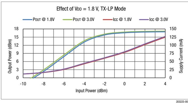
**Figure 5. Effect of Lowering VDD**
