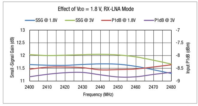
**Figure 6. Effect of Lowering VDD**
