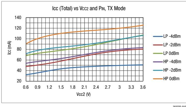
**Figure 10. I<sub>CC</sub> vs. Vcc2 and P<sub>IN</sub>**
