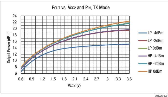
**Figure 9. P<sub>OUT</sub> vs. Vcc2 and P<sub>IN</sub>**
