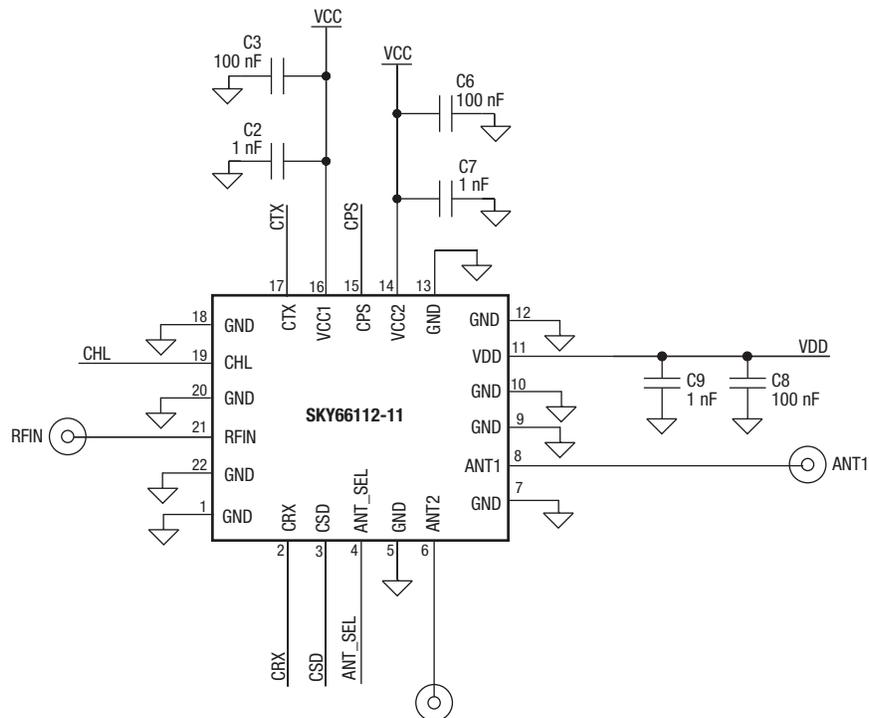
Note: The paddle should be connected to ground.
