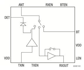
Figure 1. RFX8422S Block Diagram
