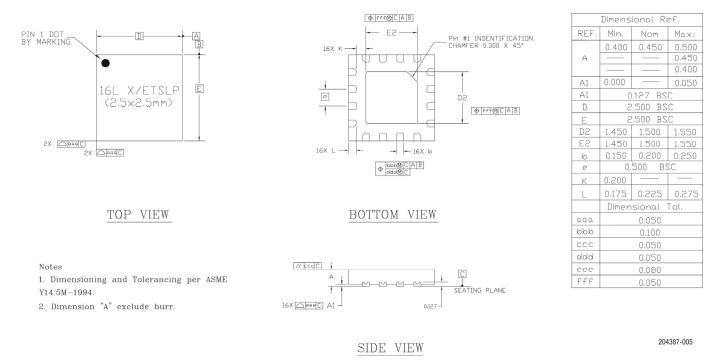
Figure 5. RFX8422S Package Dimensions
