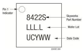
Figure 4. Typical Part Marking (Top View)
