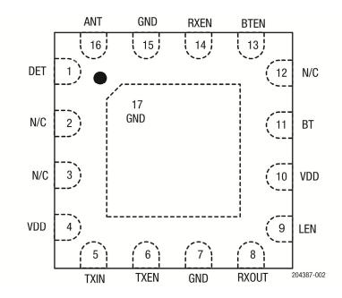
Figure 2. RFX8422S Pinout (Top View)
