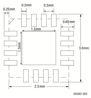
**Figure 3. RFX8422S PCB Layout Footprint**
