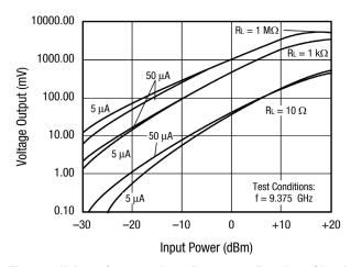
Figure 4. Voltage Output vs Input Power as a Function of Load Resistance and Bias
