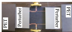
Fig. 6. Fabricated tunable DBBPF with switching function
