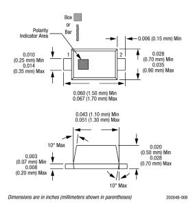
Figure 5. SC-79 Package Dimension Drawing
