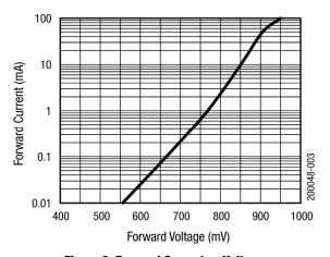
Figure 2. Forward Current vs Voltage
