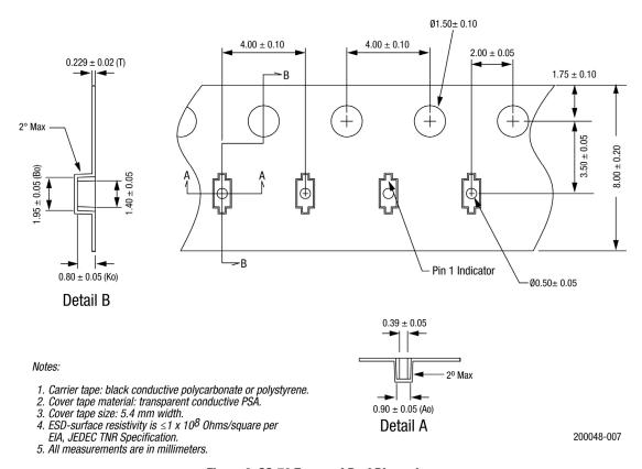
Figure 6. SC-79 Tape and Reel Dimensions
