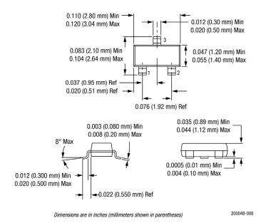
Figure 7. SOT-23 Package Dimension Drawing
