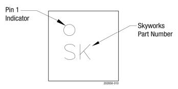
Figure 10. Typical Part Marking
