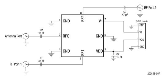
Figure 7. SKY13522-644LF Evaluation Board Schematic
