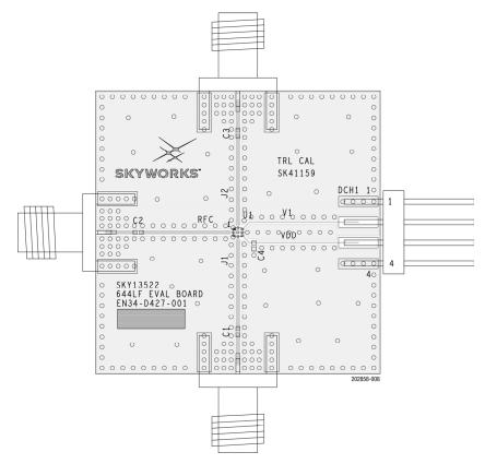
Figure 8. SKY13522-644LF Evaluation Board Assembly Diagram
