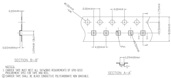
3. COVER TAPE SHALL BE TRANSPARENT CONDUCTIVE MATERIAL
