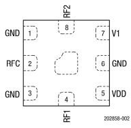
Figure 2. SKY13522-644LF Pinout (Top View)
