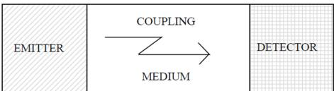
Figure 1, the basic elements of an optocoupler.
