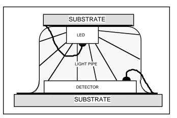
Figure 2a, side-by-side reflective coupling.
