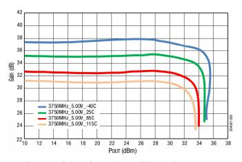
Figure 28. Gain vs Output Power (CW) over Frequency
