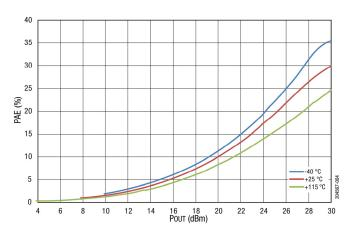
**Figure 4. PAE vs Output Power Across Temperature**
