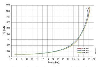
Figure 17. lop vs POUT Across Frequency @ 5 V, 25 °C
