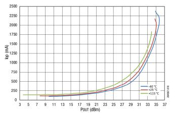
Figure 18. lop vs POUT Across Temperature @ 3500 MHz, 5V
