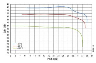
Figure 10. Gain vs POUT Across Temperature @ 3500 MHz, 5 V
