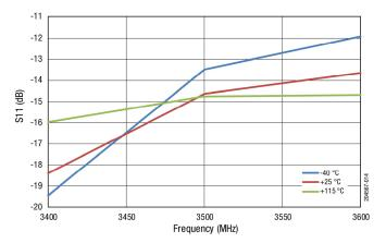
Figure 14. S11 vs Frequency Across Temperature
