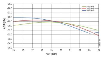
Figure 7. ACLR-5C vs POUT Across Frequency @ 5 V 25 °C
