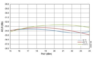
Figure 6. ACLR-1C vs Pout Across Temperature @ 3500 MHz, 5 V
