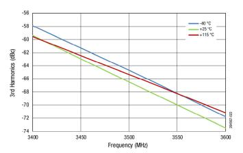
Figure 22. 3rd Harmonics @+23 dBm vs Frequency Across Temperature
