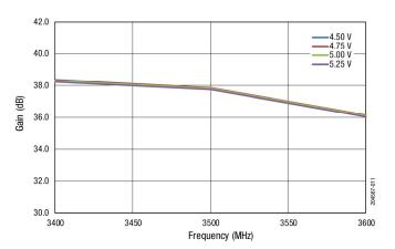
Figure 11. Gain @ +23 dBm vs Frequency Across VCC
