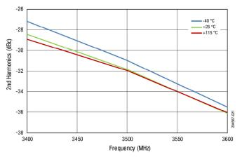
Figure 21. 2<sup>nd</sup> Harmonics @+23 dBm vs Frequency Across Temperature
