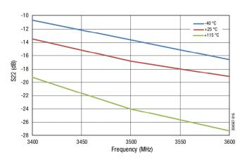
Figure 16. S22 vs Frequency Across Temperature
