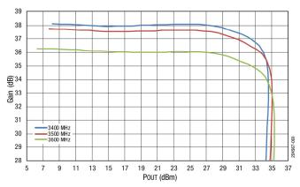
Figure 9. Gain vs POUT Across Frequency @ 5 V 25 °C
