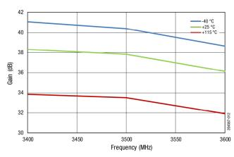
Figure 12. Gain @ +23 dBm vs Frequency Across Temperature
