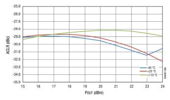
Figure 8. ACLR-5C vs POUT Across Temperature @ 3500 MHz, 5 V
