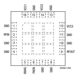
Figure 2. SKY66313-11 Pinout (Top View)
