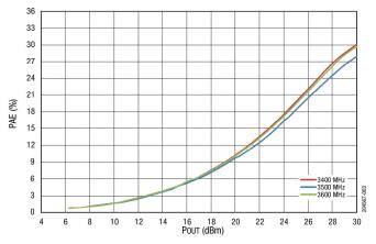
Figure 3. PAE vs Output Power (CW) Across Frequency
