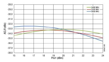
Figure 5. ACLR-1C vs POUT Across Frequency @ 5 V 25 °C
