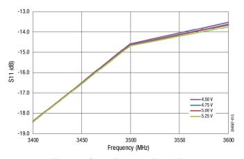
Figure 13. S11 vs Frequency Across VCC
