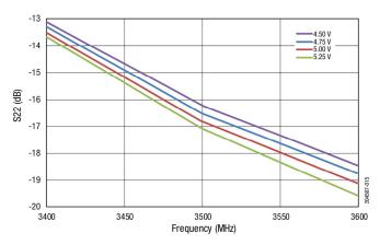
Figure 15. S22 vs Frequency Across VCC
