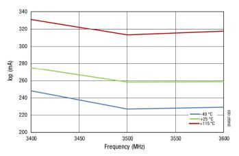
Figure 20. lop @ +23 dBm vs Frequency Across Temperature
