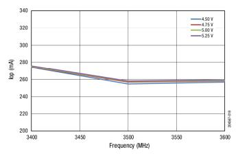
Figure 19. lop @ +23 dBm vs Frequency Across Vcc
