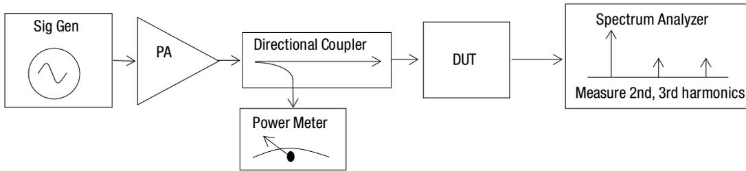
**Figure 4. Skyworks VPEAK Measurement System**
