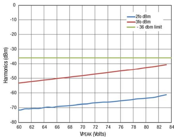
Figure 3. SKY19250-001 SPST Antenna Tuning  $V_{PEAK}$
