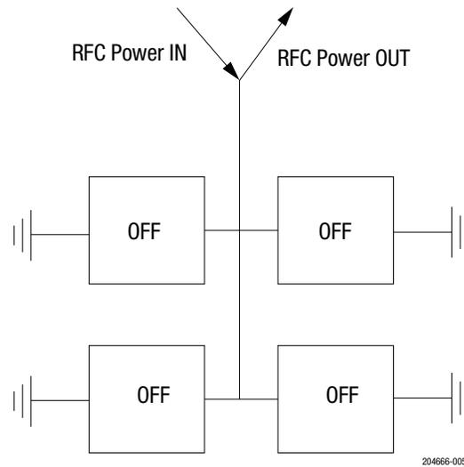
**Figure 5. VPEAK Measurement Shunt Configuration with All Arms in the “Off” State**
