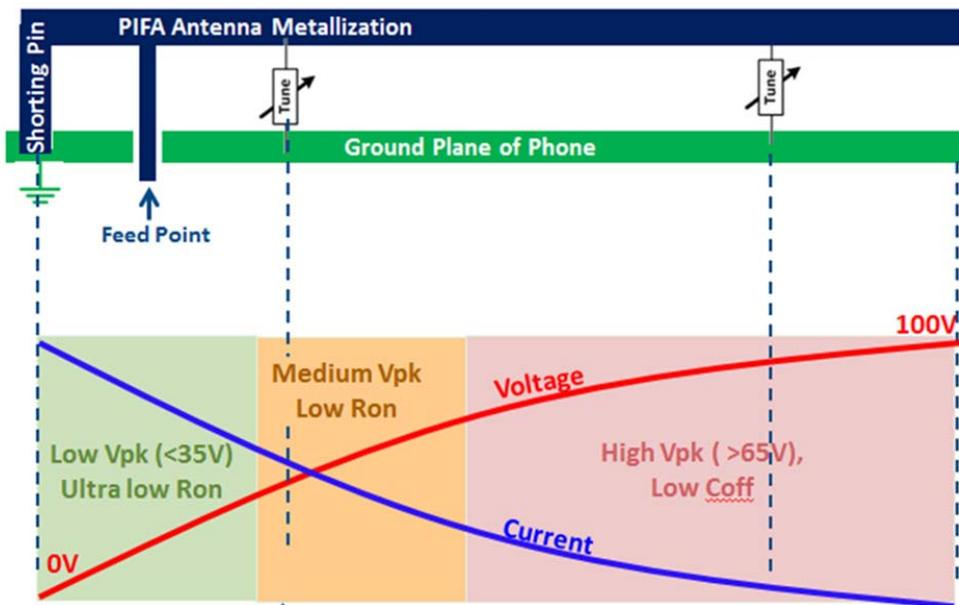
**Figure 2. Effect of the Tuning Element Location on VPEAK**
