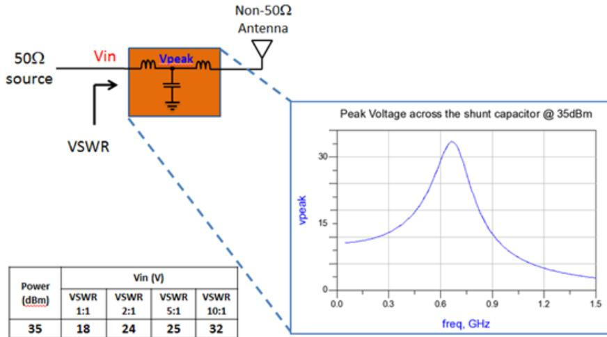
**Figure 1. Simplified Aperture Antenna (Tuner Installed Directly on Antenna Radiating Arm)**
