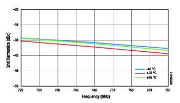
Figure 11. 2<sup>nd</sup> Harmonic vs Frequency Across Temperature @ Pout = +28 dBm (CW)
