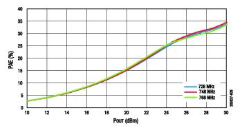
**Figure 3. PAE vs Pout Across Frequency**
