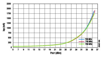
Figure 9. Operating Current vs Pout Across Frequency
