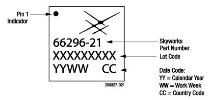
Figure 21. Typical Part Marking
