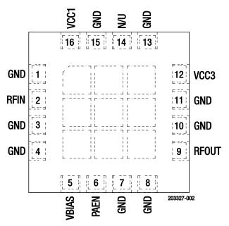
Figure 2. SKY66296-21 Pinout (Top View)
