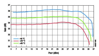
Figure 8. Gain vs Pout Across Temperature
