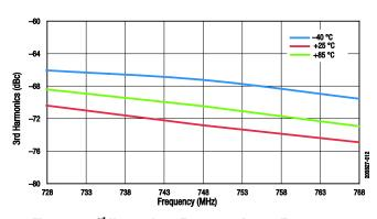
Figure 12. 3<sup>rd</sup> Harmonic vs Frequency Across Temperature @ POUT = +28 dBm(CW)
