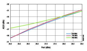
**Figure 5. ACLR vs. Pout Across Frequency**
