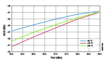
Figure 6. ACLR vs Pout Across Temperature
