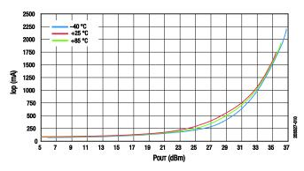
Figure 10. Operating Current vs Pout Across Temperature
