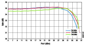
Figure 7. Gain vs Pout Across Frequency
