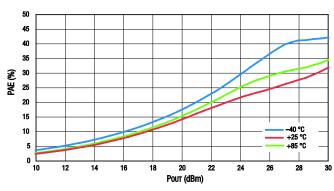
Figure 4. PAE vs Pout Across Temperature
