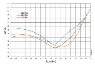
Figure 8. ACLR (5x20MHz) vs Pout Across Frequency
