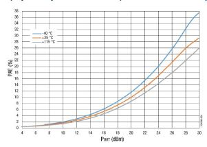
Figure 4. PAE vs Output Power (GW, 2450 MHz) Across Temperature
