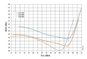
Figure 7. ACLR (1x20 MHz) vs Pout Across Frequency
