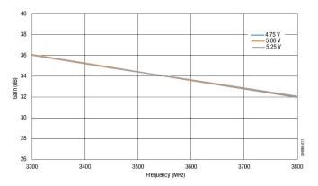
Figure 11. Gain @ +28 dBm vs Frequency Across Voltage
