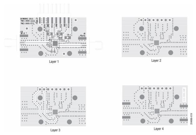
Figure 19. SKY66318-11 Evaluation Board Layer Detail
