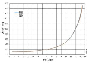
Figure 6. lop vs Pout Across Vcc @ 3450 MHz, 25  $^{\circ}$ C
