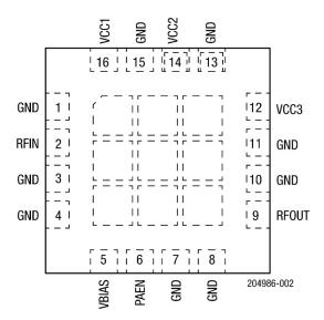
Figure 2. SKY66318-11 Pinout (Top View)
