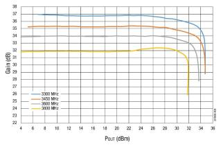
Figure 9. Gain vs Pout Across Frequency
