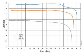
Figure 10. Gain vs Pout Across Temperature
