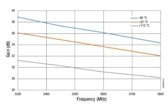
Figure 12. Gain @ +28 dBm vs Frequency Across Temperature
