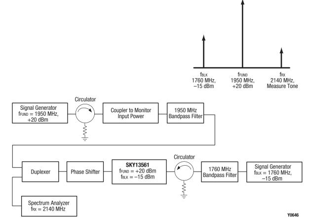
Figure 3. 3<sup>rd</sup> Order Intermodulation Test Setup
