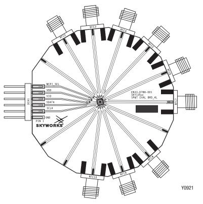
Figure 8. SKY13561-670LF Evaluation Board Assembly Diagram
