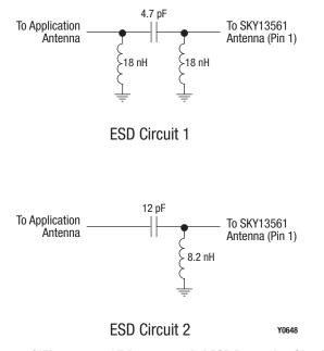
Figure 7. SKY13561-670LF Recommended ESD Protection Circuits
