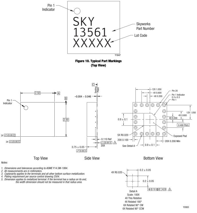
Figure 11. SKY13561-670LF 20-Pin QFN Package Dimensions
