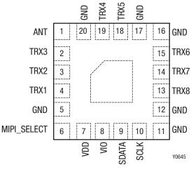
Figure 2. SKY13561-670LF Pinout – 20-Pin QFN (Top View)
