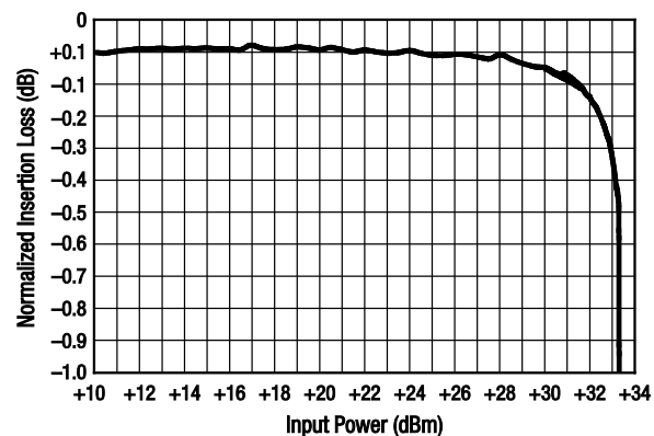
Figure 6. Normalized Insertion Loss vs Input Power
