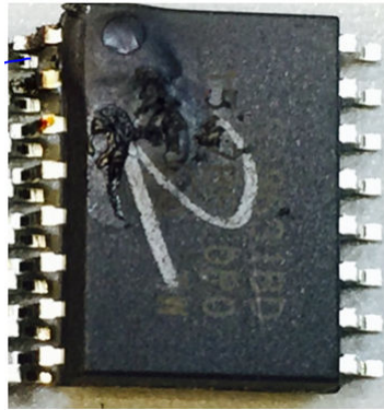
Figure 6.1. Visible Package Damage after EOS1-Induced Failure
