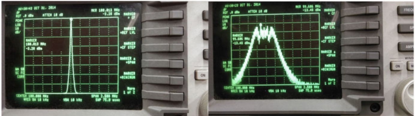
Figure 3.1. EMI Reduction due to -0.5% Down Spread on a 100 MHz Clock Used for PCIe Applications
