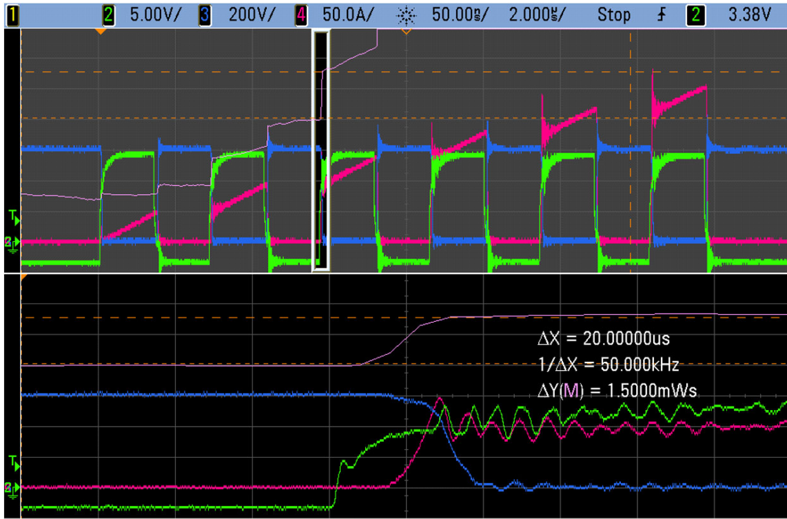
Figure 10. EON Loss I_{DS} = 100A , L_O = 18\mu H , ( V_{DS} = 600V )
