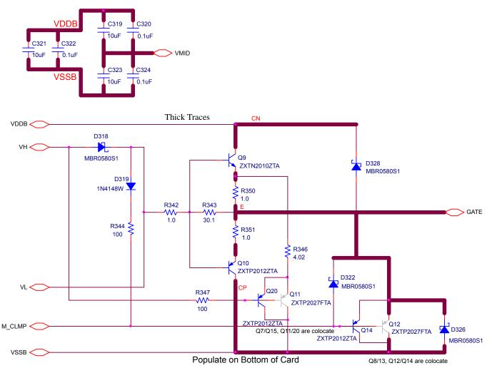
Figure 1.6. Low-Side Current Booster Circuit
