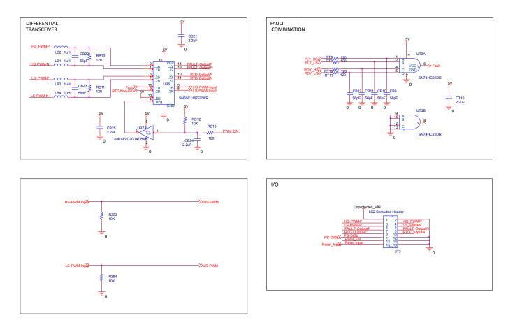
Figure 1.2. Low-Voltage Signals and I/O
