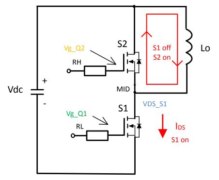
Figure 4.1. Switching Loss Test Circuit
