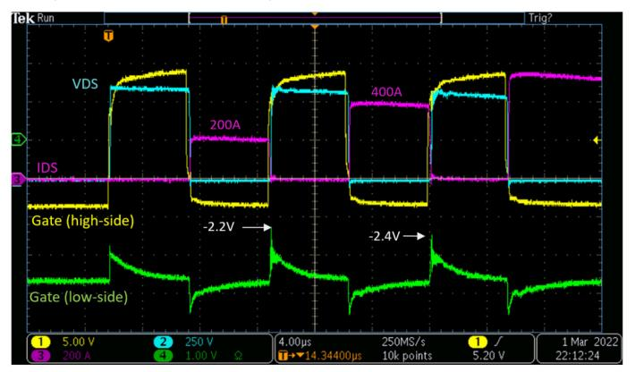
Figure 3.2. Crosstalk Test RH = RL = 1  $\Omega$ , V<sub>DS</sub> = 600 V, Lo = 14  $\mu$ H
