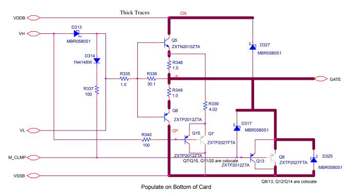
Figure 1.5. High-Side Current Booster Circuit
