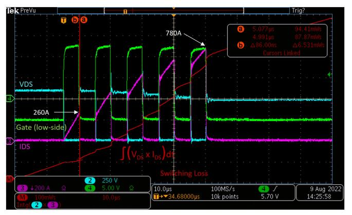
Figure 4.2. Switching Loss Test  $R_H = R_L = 1 \Omega$ , Lo = 14 µH, IDS = 0 A-780 A, VDS = 600 V
