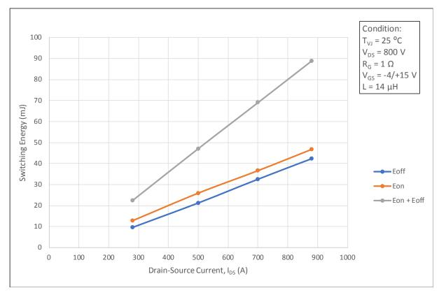
Figure 4.6. Switching Loss vs. Drain Current RH = RL = 1  $\Omega$  (V<sub>DS</sub> = 800 V)
