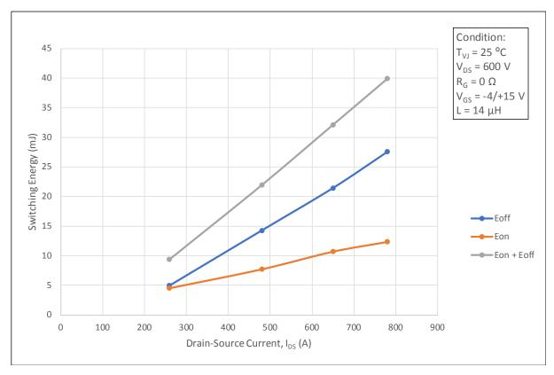
Figure 4.12. Switching Loss vs. Drain Current  $R_H = R_L = 0 \Omega (V_{DS} = 600 V)$
