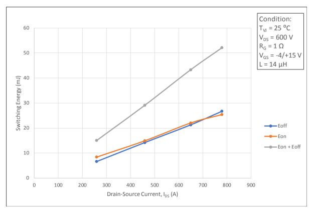
Figure 4.4. Switching Loss vs. Drain Current RH = RL = 1  $\Omega$  (V<sub>DS</sub> = 600 V)
