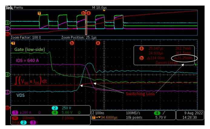
Figure 4.3. Switching Eoff Loss  $R_H = R_L = 1 \Omega$ , IDS = 650 A, Lo = 14  $\mu$ H, (VDS = 600 V)
