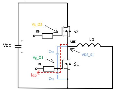
Figure 3.1. Crosstalk Test Circuit
