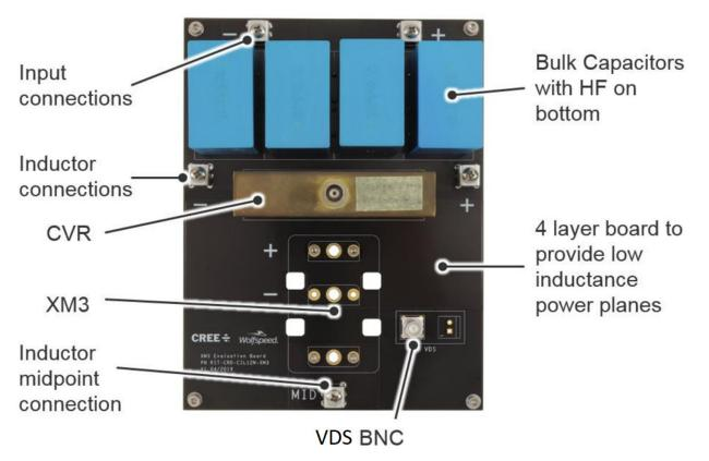
Figure 1.10. Wolfspeed's KIT-CRD-CIL12N-XM3 CIL Evaluation Board
