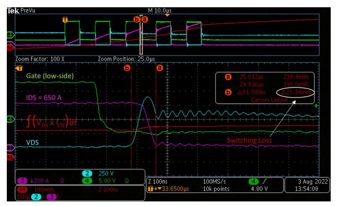
Figure 4.11. Switching Eoff Loss  $R_H = R_L = 0 \Omega$ , Lo = 14  $\mu$ H, IDS = 650 A, VDS = 600 V
