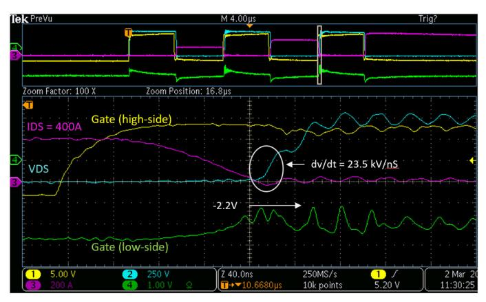
Figure 3.9. Crosstalk Test RH = RL = 0  $\Omega$ , V<sub>DS</sub> = 800 V, Lo = 14  $\mu$ H (Zoomed)
