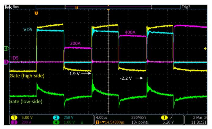
Figure 3.6. Crosstalk Test RH = RL = 0  $\Omega$ , V<sub>DS</sub> = 600 V, Lo = 14 $\mu$ H
