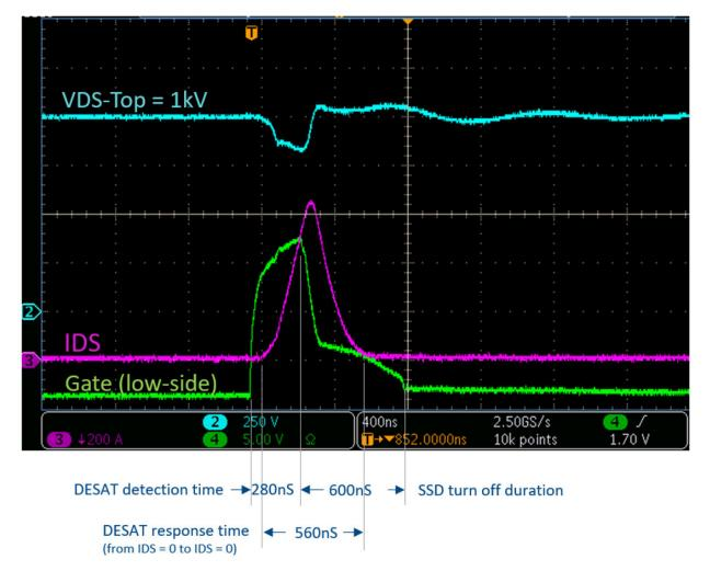
Figure 2.4. Si828x 560 ns DESAT response time with RI = 2.2 k $\Omega$ , RH = RL = 1  $\Omega$ , RSS = 1  $\Omega$
