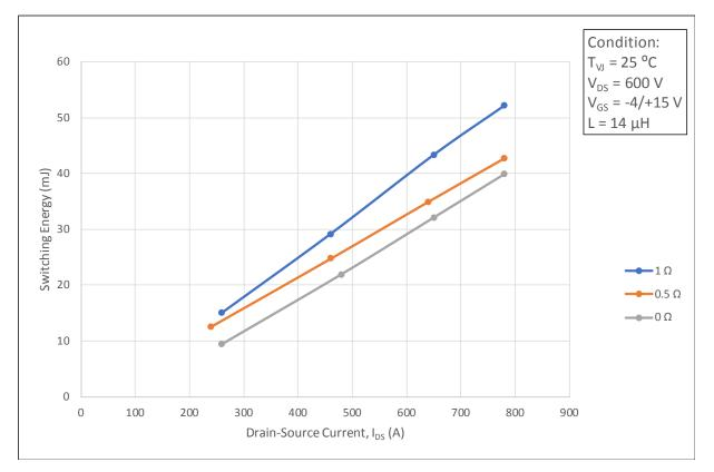
Figure 4.15. Total Switching Loss vs. Rg ( $R_H = R_L$ ),  $V_{DS} = 600 V$
