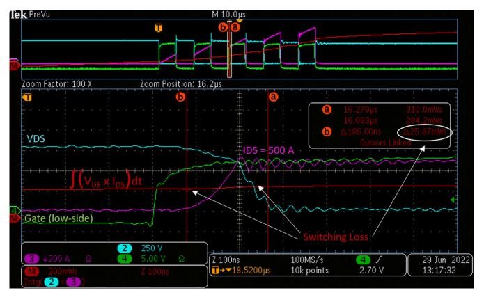
Figure 4.5. Switching Eon Loss  $R_{H}$  =  $R_{L}$  = 1  $\Omega,$  Lo = 14  $\mu H,$  IDS = 500 A, VDS = 800 V
