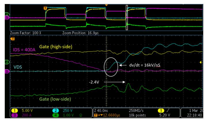
Figure 3.5. Crosstalk Test RH = RL = 1  $\Omega$ , V<sub>DS</sub> = 800 V, I<sub>DS</sub> = 400A, Lo = 14  $\mu$ H (Zoomed)
