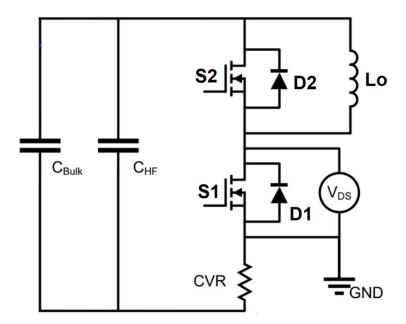
Figure 1.9. Wolfspeed's KIT-CRD-CIL12N-XM3 Simplified Schematic
