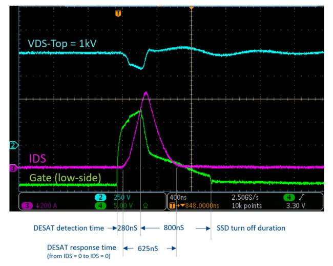
Figure 2.5. Si828x 625 ns DESAT response time with RI = 2.2 k $\Omega$ , RH = RL = 1  $\Omega$ , RSS = 4.02  $\Omega$
