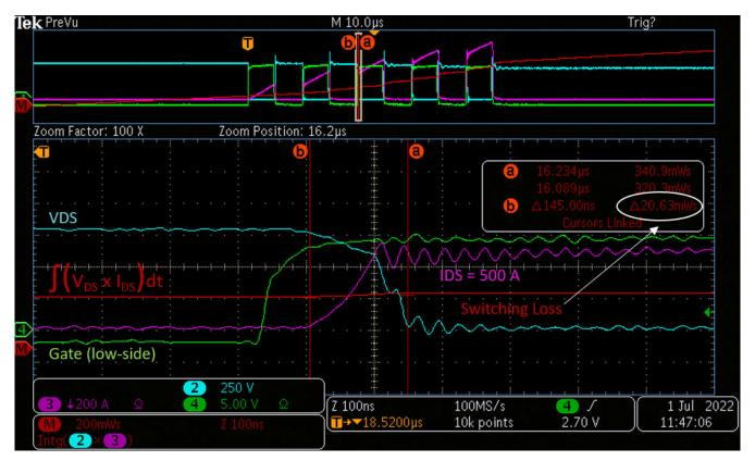
Figure 4.9. Switching Eon Loss  $R_{H}$  =  $R_{L}$  = 0.5  $\Omega,$  Lo = 14  $\mu H,$  IDS = 500 A, VDS = 800 V
