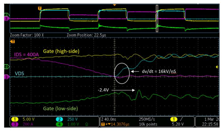
Figure 3.3. Crosstalk Test RH = RL = 1  $\Omega$ , V<sub>DS</sub> = 600 V, Lo = 14 $\mu$ H, I<sub>DS</sub> = 400 A (Zoomed)
