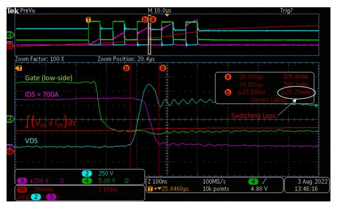
Figure 4.13. Switching Eoff Loss  $R_H = R_L = 0 \Omega$ , Lo = 14  $\mu$ H, IDS = 700 A, VDS = 800 V
