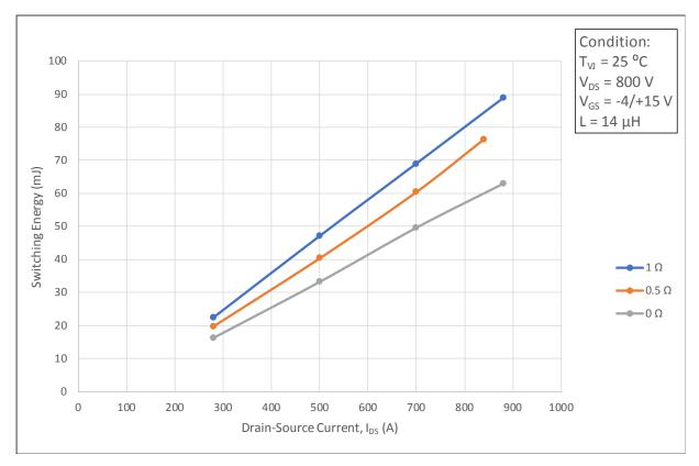
Figure 4.16. Total Switching Loss vs. Rg (RH = RL), V<sub>DS</sub> = 800 V
