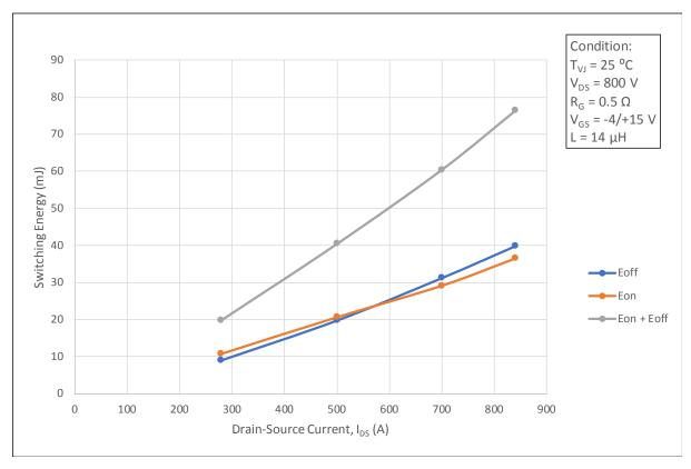
Figure 4.10. Switching Loss vs. Drain Current RH = RL = 0.5  $\Omega$  (V<sub>DS</sub> = 800 V)
