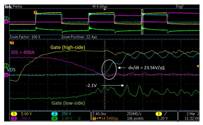
Figure 3.7. Crosstalk Test RH = RL = 0  $\Omega$ , V<sub>DS</sub> = 600 V, I<sub>DS</sub> = 400A, Lo = 14  $\mu$ H (Zoomed)
