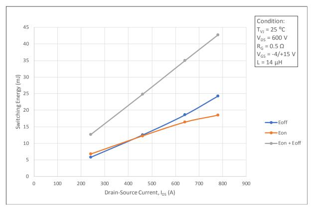
Figure 4.8. Switching Loss vs. Drain Current RH = RL = 0.5  $\Omega$  (V<sub>DS</sub> = 600 V)
