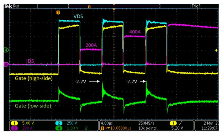
Figure 3.8. Crosstalk Test RH = RL = 0  $\Omega$ , V<sub>DS</sub> = 800 V, Lo = 14  $\mu$ H
