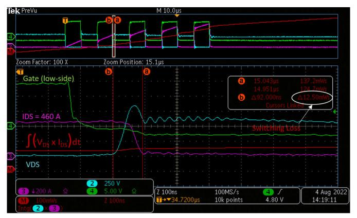
Figure 4.7. Switching Eoff Loss  $R_{H}$  =  $R_{L}$  = 0.5  $\Omega,$  Lo = 14  $\mu H,$  IDS = 460 A, VDS = 600 V
