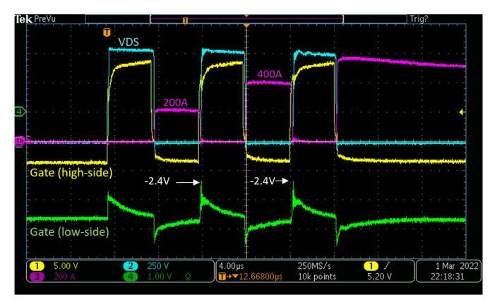
Figure 3.4. Crosstalk Test RH = RL = 1  $\Omega$ , V<sub>DS</sub> = 800 V, Lo = 14 $\mu$ H
