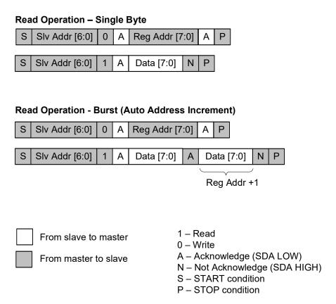
Figure 6. I<sup>2</sup>C Read Operation
