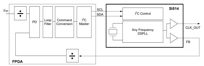
Figure 3. All-Digital PLL Application Using Si514 with Dual CMOS Output
