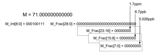
Figure 4. Output Frequency Change When Toggling M\_Frac[N], M=71
