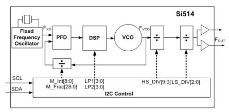
Figure 1. Block Diagram of Si514
