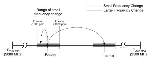
Programming a new center frequency requires a VCO calibration and the output should be squelched
