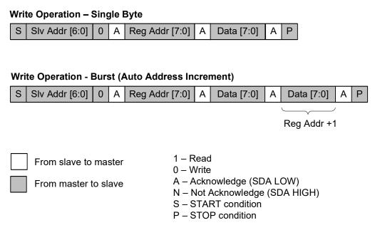
Figure 5. I<sup>2</sup>C Write Operation
