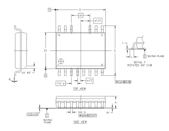
Figure 7.4. 14-Pin Small Outline Integrated Circuit (SOIC) Package
