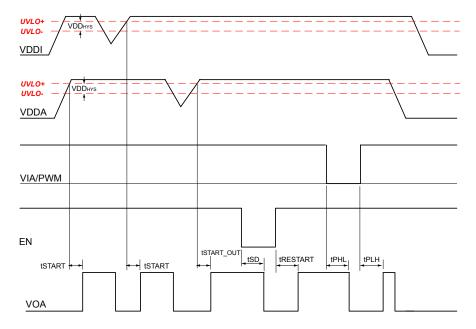
Figure 2.3. Si823H2/4/5/7/9 Device Behavior During Normal Operation and Shutdown
