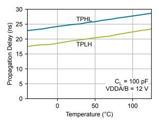
Figure 4.6. Propagation Delay vs. Temperature
