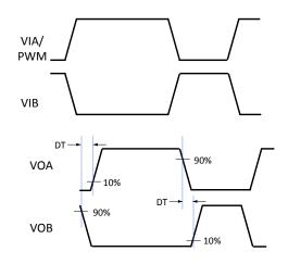
Figure 2.7. Dead Time Waveforms for High-Side/Low-Side Drivers
