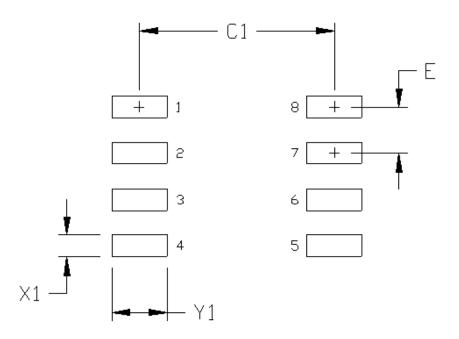
Figure 8.1. 8-Pin Narrow Body SOIC Land Pattern
