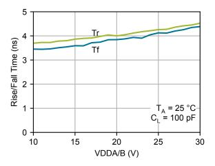
Figure 4.2. Rise/Fall Time vs. Supply Voltage
