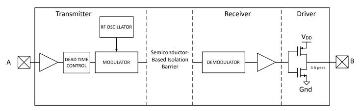
Figure 2.1. Simplified Channel Diagram
