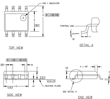
Figure 7.1. 8-Pin Narrow Body SOIC Package
