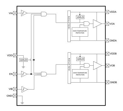
Figure 5.8. Si823H5/7 Dual Isolated Drivers with EN
