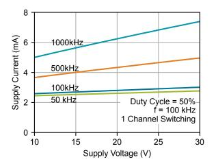
Figure 4.8. Supply Current vs. Supply Voltage (C<sub>L</sub> = 0 pF)
