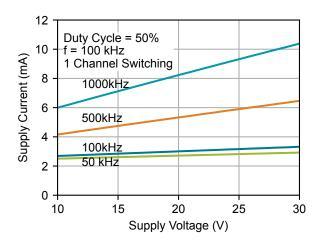
Figure 4.9. Supply Current vs. Supply Voltage (C<sub>L</sub> = 100 pF)
