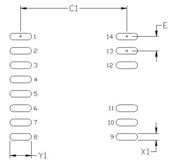
Figure 8.4. 14-Pin WB SOIC Land Pattern
