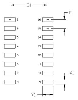
Figure 8.3. 16-Pin Narrow Body SOIC PCB Land Pattern
