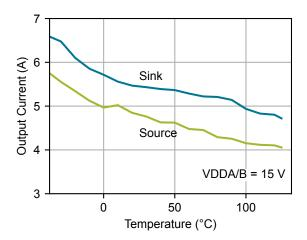
Figure 4.11. Peak Output Current vs. Temperature
