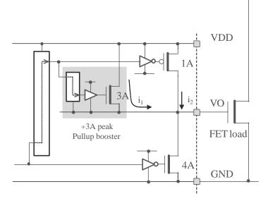
Figure 2.8. Pull-Up Booster Simplified Architecture
