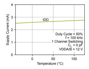
Figure 4.7. Supply Current vs. Temperature
