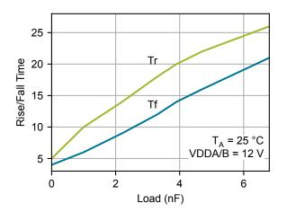
Figure 4.4. Rise/Fall Time vs. Load
