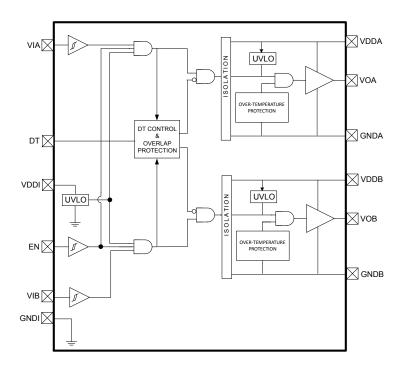
Figure 5.3. Si823H2 HS/LS Isolated Drivers with EN
