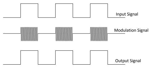
Figure 2.2. Modulation Scheme
