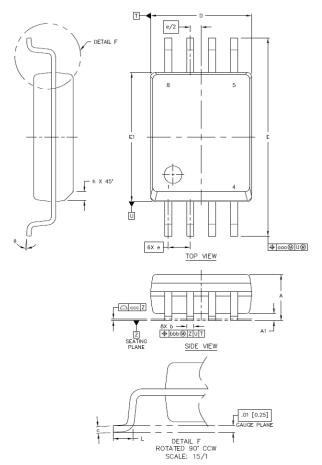
Figure 7.2. 8-Pin Wide Body Stretched SOIC Package
