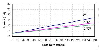
Figure 10. Si8442 Typical V<sub>DD1</sub> or V<sub>DD2</sub> Supply Current vs. Data Rate 5, 3.3, and 2.70 V Operation (15 pF Load)
