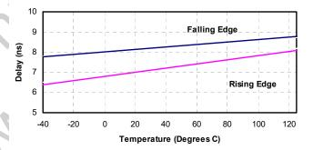
Figure 12. Propagation Delay vs. Temperature
