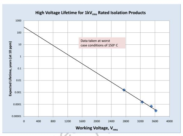
Figure 13. Si84xx Time-Dependent Dielectric Breakdown
