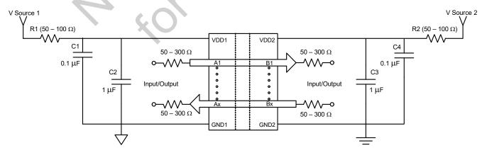
Figure 8. Recommended Bypass Components for the Si84xx Digital Isolator Family
