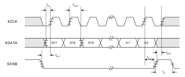
Figure 2. Serial Interface Timing Diagram
