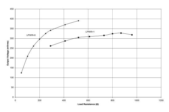
Figure 18. Typical IF Output Voltage vs. Load Resistance at 550 MHz
