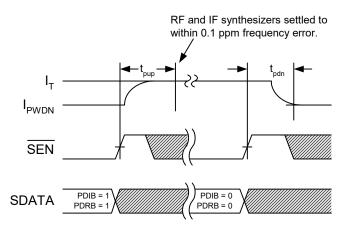
Figure 4. Software Power Management Timing Diagram
