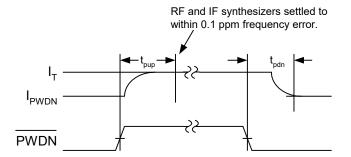
Figure 5. Hardware Power Management Timing Diagram
