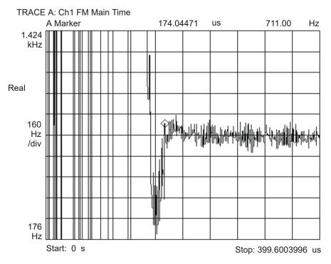
Figure 6. Typical Transient Response RF1 at 1.6 GHz with 200 kHz Phase Detector Update Frequency
