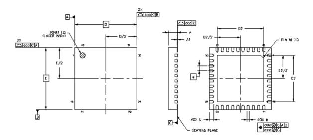
Figure 7.2. 40-Pin Quad Flat No-Lead (QFN)
