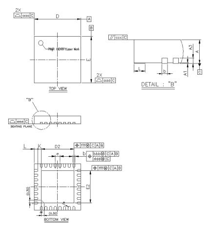
Figure 7.3. 32-Pin Quad Flat No-Lead (QFN)
