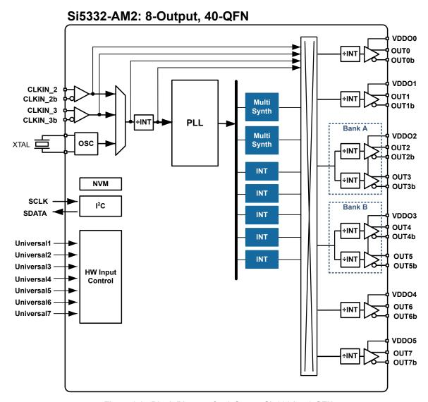
Figure 3.2. Block Diagram for 8-Output Si5332 in 40-QFN
