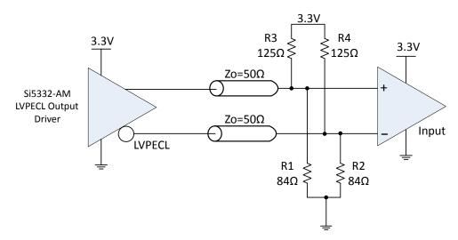
Figure 3.8. 3.3 V LVPECL Output Termination, Option 2
