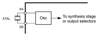
Figure 3.4. External Reference Input (XA/XB)
