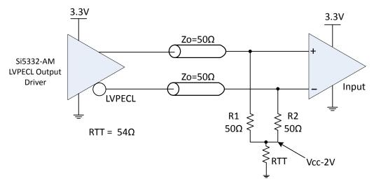
Figure 3.7. 3.3 V LVPECL Output Termination, Option 1
