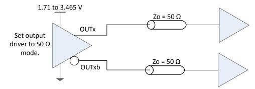
Figure 3.13. LVCMOS Output Termination Example, Option 1
