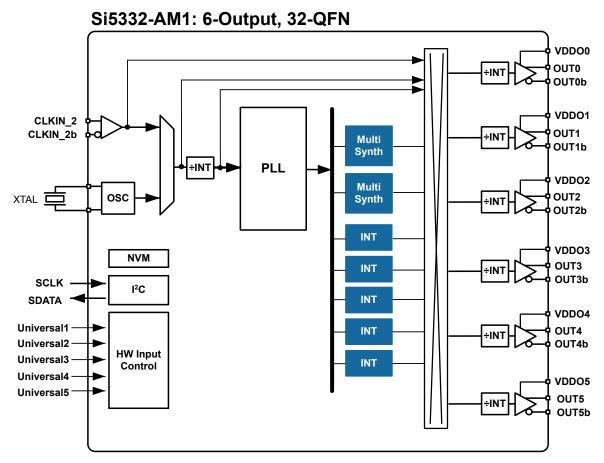
Figure 3.3. Block Diagram for 6-Output Si5332 in 32-QFN
