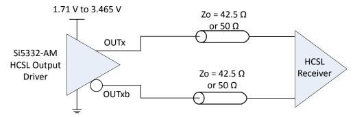
Figure 3.11. HCSL Internal Termination Mode
