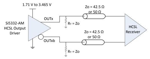
Figure 3.12. HCSL External Termination Mode
