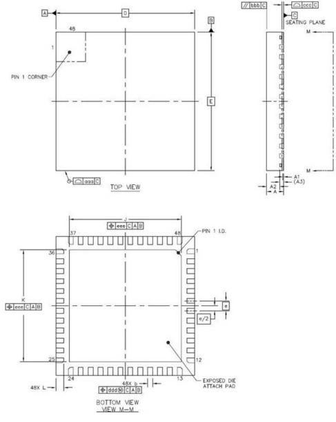
Figure 7.1. 48-Pin Quad Flat No-Lead (QFN)
