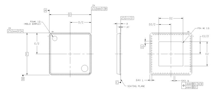
Figure 9.1. Si5386 9x9 mm 64-QFN Package Diagram
