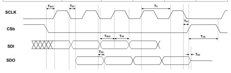
Figure 5.2. 4-Wire SPI Serial Interface Timing
