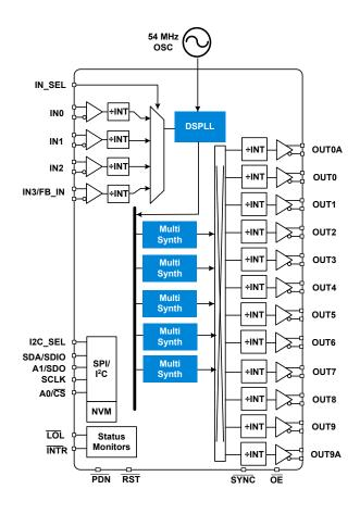
Figure 6.1. Si5386 Block Diagram
