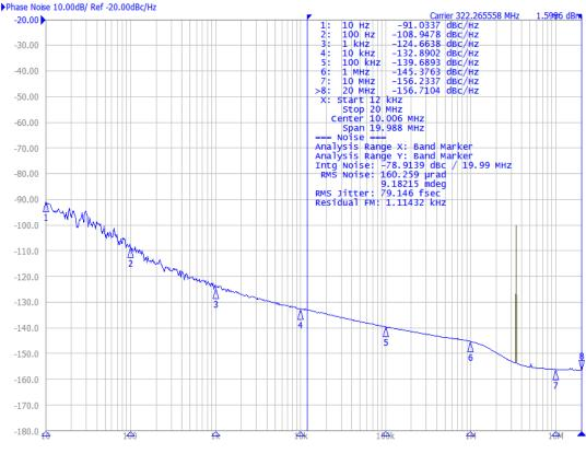
Figure 7.3. f<sub>IN</sub> = 322.265625 MHz, f<sub>OUT</sub> = 322.265625 MHz
