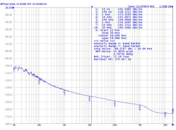
Figure 7.1. f<sub>IN</sub> = 156.25 MHz, f<sub>OUT</sub> = 122.88 MHz
