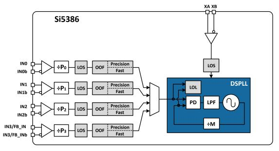
Figure 3.4. Si5386 Fault Monitors (Grade A)
