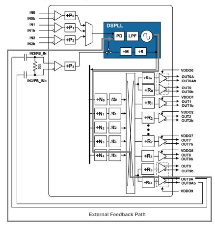
Figure 3.12. Si5386 Zero Delay Mode Setup
