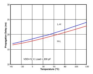
Figure 2.10. Propagation Delay vs. Temperature
