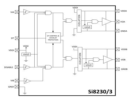
Figure 2.1. Si8230/3 Two-Input High-Side/Low-Side Isolated Drivers
