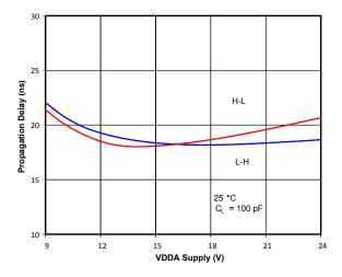
Figure 2.7. Propagation Delay vs. Supply Voltage
