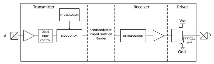
Figure 2.4. Simplified Channel Diagram
