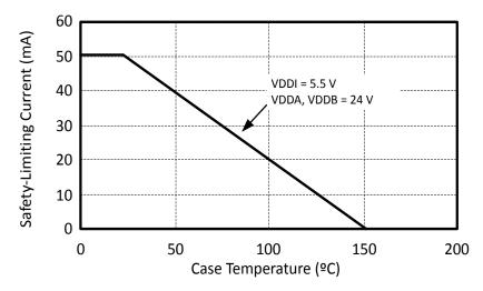
Figure 3.4. WB SOIC, NB SOIC, 14 LD LGA/QFN Thermal Derating Curve, Dependence of Safety Limiting Values with Case Temperature per VDE 0884-10
