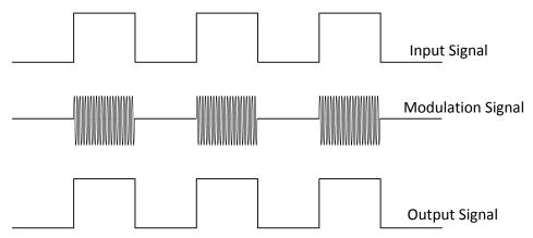
Figure 2.5. Modulation Scheme
