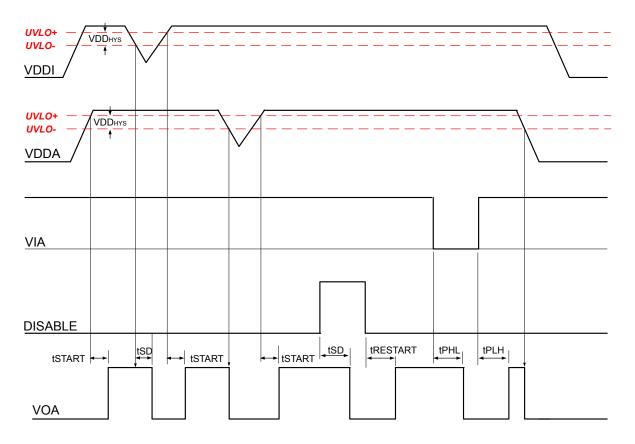
Figure 2.30. Device Behavior during Normal Operation and Shutdown
