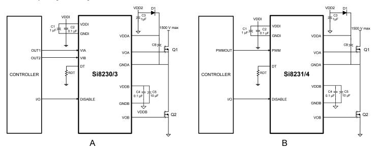
Figure 4.1. Si823x in Half-Bridge Application
