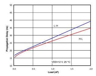
Figure 2.9. Propagation Delay vs. Load
