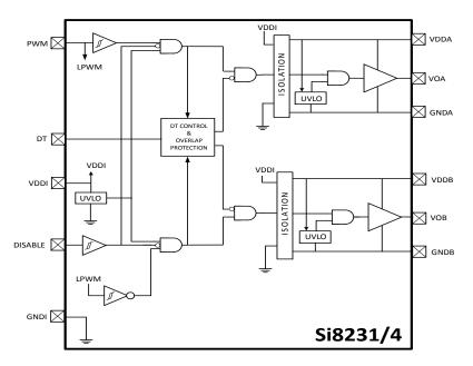
Figure 2.2. Si8231/4 Single-Input High-Side/Low-Side Isolated Drivers
