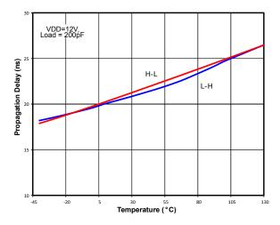
Figure 2.22. Propagation Delay vs. Temperature
