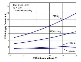
Figure 2.24. Supply Current vs. Supply Voltage
