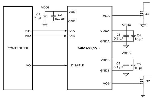
Figure 4.2. Si8232/5/7/8 in a Dual Driver Application
