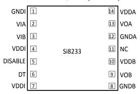
Table 5.4. Si8233 Two-Input HS/LS Isolated Driver (14 LD LGA and QFN)
