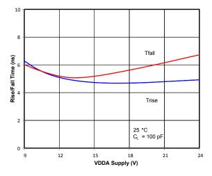
Figure 2.6. Rise/Fall Time vs. Supply Voltage
