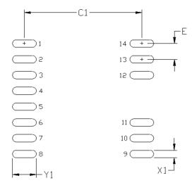
Figure 7.2. 14-Pin WB SOIC Land Pattern
