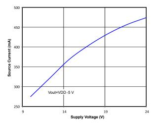
Figure 2.14. Output Source Current vs. Supply Voltage
