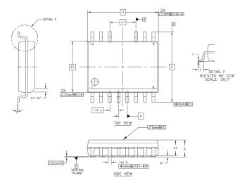
Figure 6.2. Si823x 14-pin WB SOIC Outline
