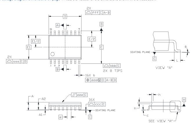
Figure 6.1. 16-Pin Wide Body SOIC
