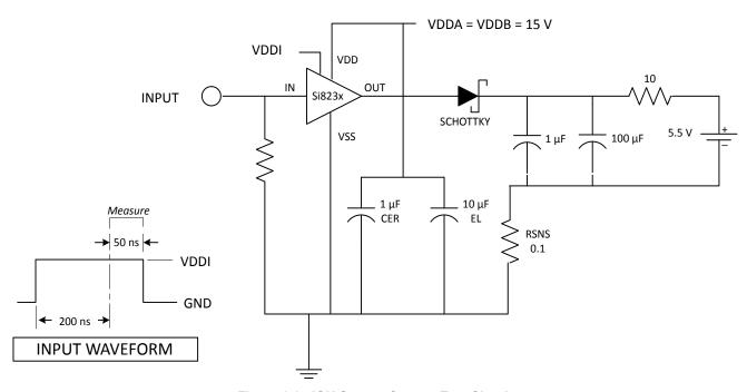
Figure 3.2. IOH Source Current Test Circuit
