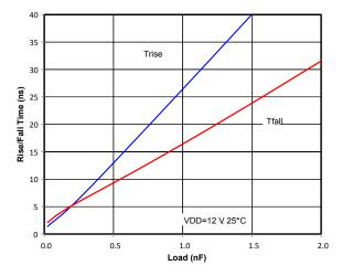
Figure 2.8. Rise/Fall Time vs. Load
