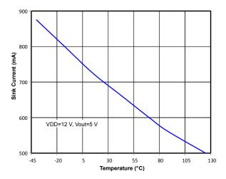
Figure 2.17. Output Sink Current vs. Temperature
