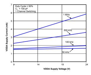
Figure 2.13. Supply Current vs. Supply Voltage
