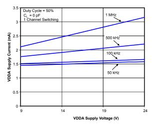
Figure 2.12. Supply Current vs. Supply Voltage
