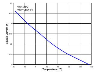
Figure 2.27. Output Source Current vs. Temperature
