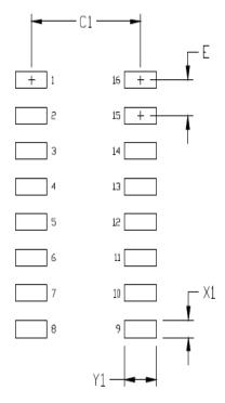
Figure 7.3. 16-Pin Narrow Body SOIC PCB Land Pattern
