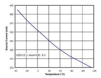
Figure 2.15. Output Source Current vs. Temperature
