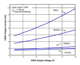
Figure 2.25. Supply Current vs. Supply Voltage
