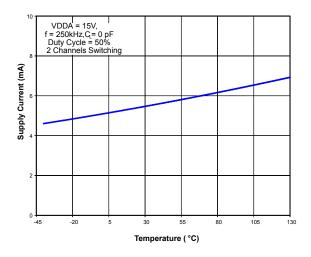
Figure 2.23. Supply Current vs. Temperature
