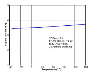
Figure 2.11. Supply Current vs. Temperature
