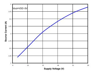
Figure 2.26. Output Source Current vs. Supply Voltage
