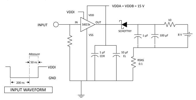
Figure 3.1. IOL Sink Current Test Circuit
