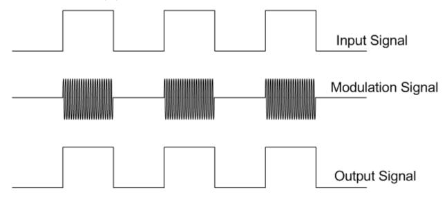
Figure 2.2. Modulation Scheme
