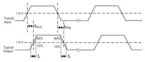
Figure 4.2. Propagation Delay Timing
