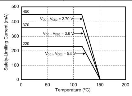
Figure 4.4. (WB SOIC-16) Thermal Derating Curve, Dependence of Safety Limiting Values with Case Temperature per DIN EN 60747-5-5/VDE 0884-10, as Applies
