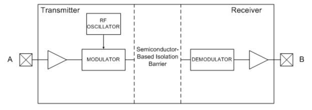
Figure 2.1. Simplified Channel Diagram
