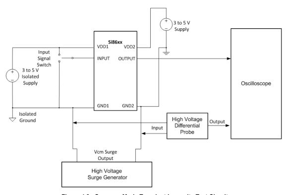
Figure 4.3. Common-Mode Transient Immunity Test Circuit
