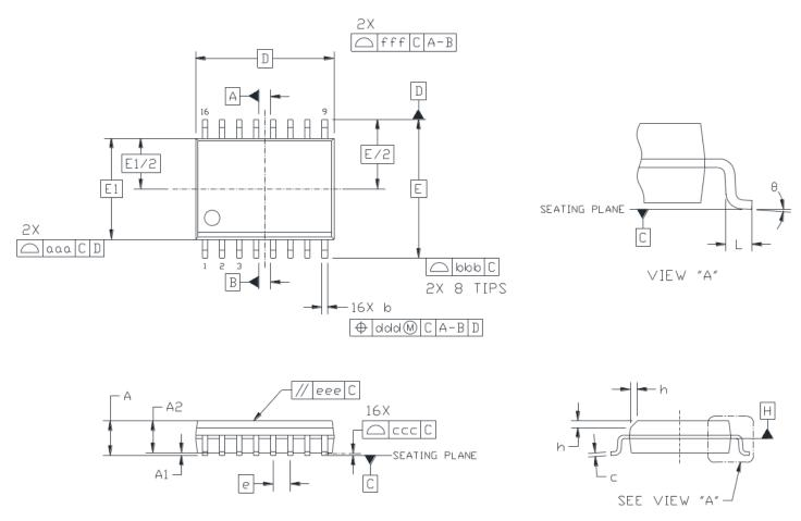
Figure 6.1. 16-Pin Wide Body SOIC
