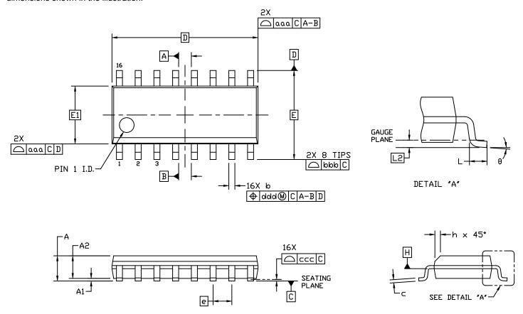
Table 8.1. 16-Pin Narrow Body SOIC Package Diagram Dimensions 1, 2, 3, 4
