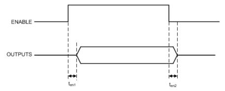
Figure 4.1. ENABLE Timing Diagram
