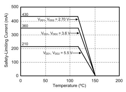
Figure 4.5. (NB SOIC-16) Thermal Derating Curve, Dependence of Safety Limiting Values with Case Temperature per DIN EN 60747-5-5/VDE 0884-10, as Applies
