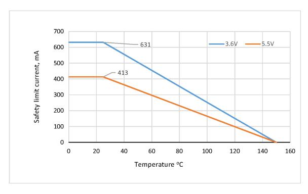
Figure 39. WB SOIC-16/20 Thermal Derating Curve (Dependence of Safety Limiting Values)
