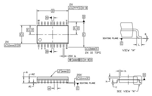
Figure 41. 20-Pin Wide-Body SOIC Package Diagram
