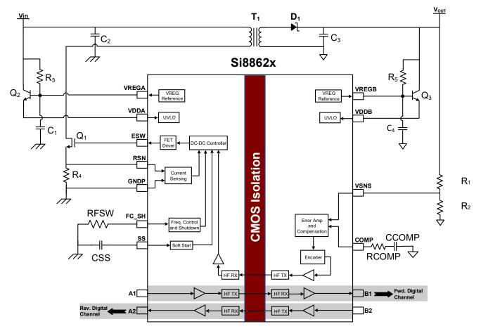
Figure 10. Si886xx Block Diagram: Up to 24 V Input to up to 24 V Output
