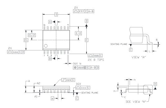
Figure 40. 16-Pin Wide-Body SOIC Package Diagram
