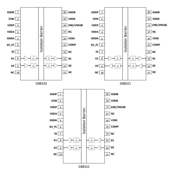
Figure 2. Si8832x Pin Configurations
