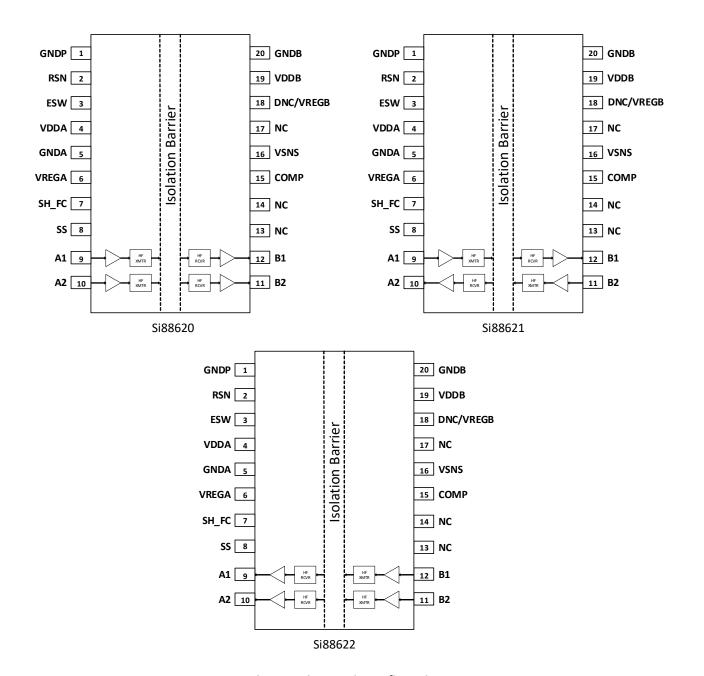
Figure 4. Si8862x Pin Configurations
