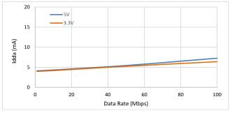
Figure 13. Si88621 Typical V<sub>DDA</sub> Supply Current vs. Data Rate Using V<sub>REGA</sub> (4.3 V)
