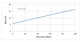
Figure 14. Si88621 Typical V<sub>DDB</sub> Supply Current vs. Data Rate (5 V and 3.3 V Operation)
