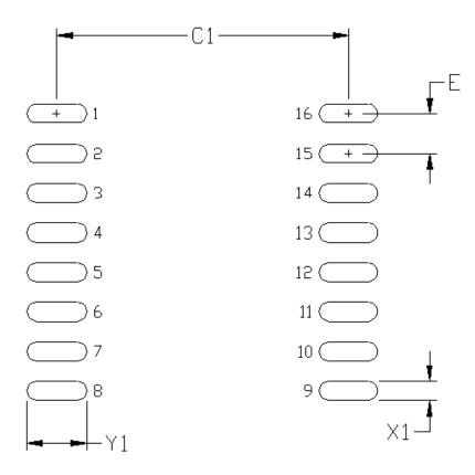
Figure 42. 16-Pin Wide-Body SOIC Land Pattern Drawing
