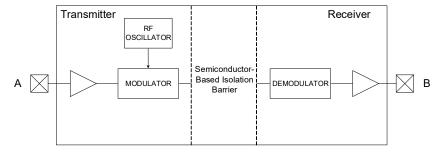
Figure 5. Simplified Si88xx Channel Diagram
