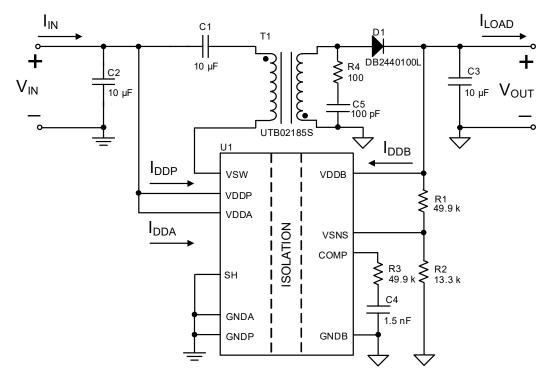
Figure 36. Measurement Circuit for Converter Efficiency and Regulation for Si882xx, Si883xx
