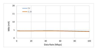
Figure 15. Si88622 Typical  $V_{DDA}$  Supply Current vs. Data Rate Using  $V_{REGA}$  (4.3 V)
