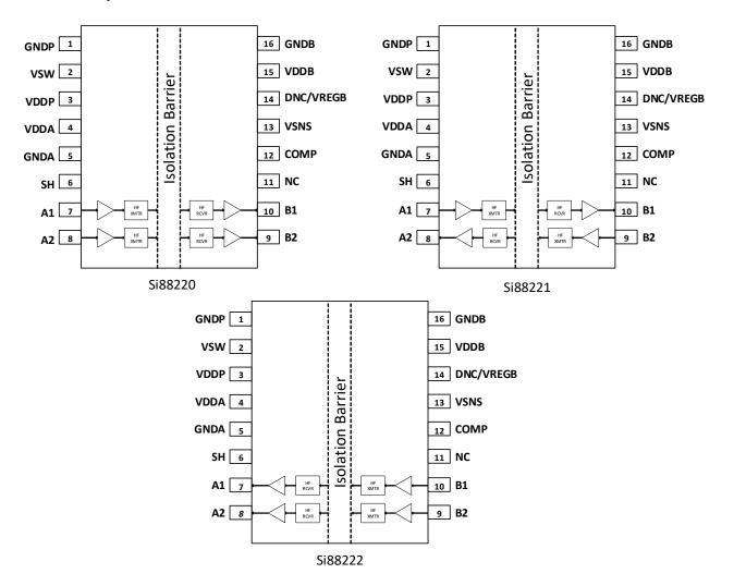
Figure 1. Si8822x Pin Configurations
