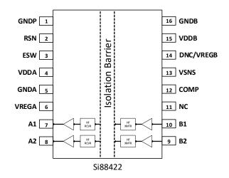
Figure 3. Si8842x Pin Configurations
