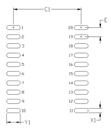
Figure 43. 20-Pin SOIC PCB Land Pattern Drawing
