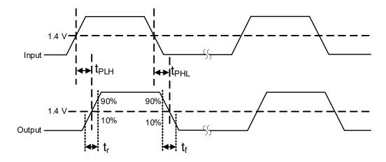
Figure 35. Propagation Delay Timing for Digital Channels
