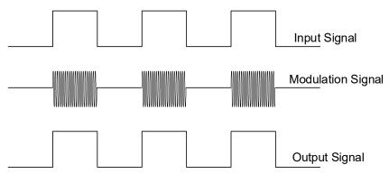
Figure 6. Modulation Scheme
