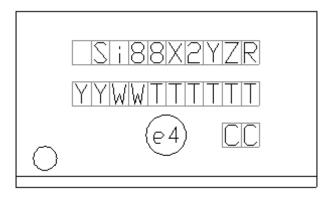
Figure 45. 20-Pin Wide-Body SOIC Top Marking
