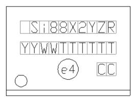
Figure 44. 16-Pin Wide-Body SOIC Top Marking
