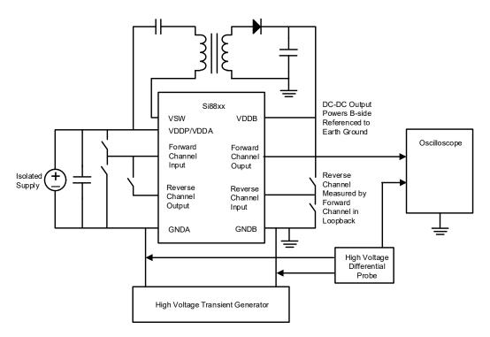
Figure 38. Common-Mode Transient Immunity Test Circuit
